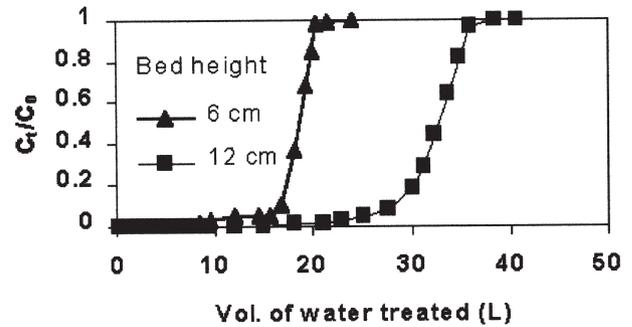
**Fig. 10.** Effect of bed height on shape of breakthrough curve ( $2 \text{ mL min}^{-1}$ ,  $C_0$  0.5 mg/L).
