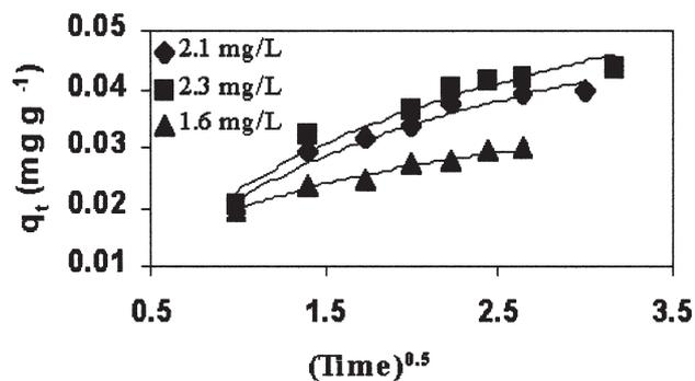
**Fig. 8.** Estimation of intra particle diffusion rate constants (pH 12.0; adsorbent dose 50 g L<sup>-1</sup>; temperature 298 K).
