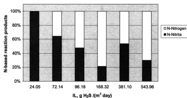
**Fig. 7.** The variation of the ratio of N-degradation products as a function of H<sub>2</sub>S loading rate.
