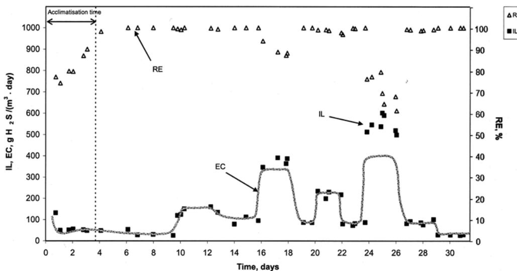
**Fig 3.** Variation of  $H_2S$  removal efficiency (RE),  $H_2S$  loading rate (IL), and biofilter elimination capacity (EC) as a function of time.
