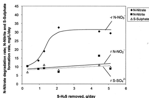
**Fig. 5.** Variation of N-nitrate degradation rate, and N-nitrite and S-sulphate formation rates as a function amount of daily hydrogen sulphide removed.
