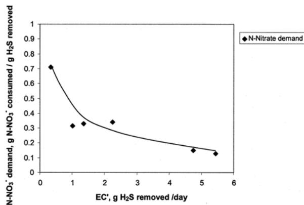
Fig. 8. Variation of nitrate demand as a function of biofilter elimination capacity.
