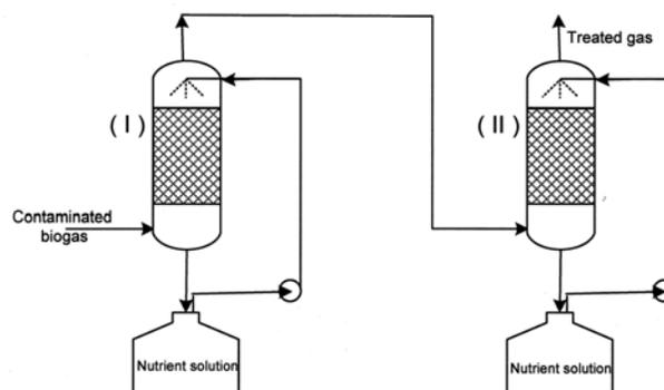
**Fig. 2.** Simplified diagram of two bioreactors operating in series. (I): Biotrickling filter packed with plastic fibres (0.012 m<sup>3</sup>); (II): Biotrickling filter packed with plastic fibres and volcanic rocks (0.014 m<sup>3</sup>). Hatched area, packing bed: (I), 0.68-m media height; (II), 0.80-m media height.
