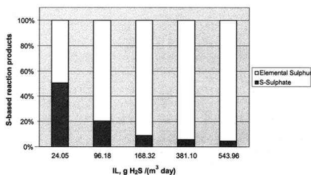
**Fig. 6.** The variation of the ratio of S-degradation products as a function of H<sub>2</sub>S loading rate.
