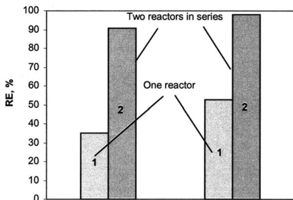
**Fig. 9.** Increasing H<sub>2</sub>S removal efficiency by operating two reactors in series. Reactor(I): Biotrickling filter packed with plastic fibres (0.012-m<sup>3</sup>bed volume, Soreanu et al. 2007); Reactor(II): Biotrickling filter packed with rocks and plastic fibres (0.014-m<sup>3</sup>bed volume).
