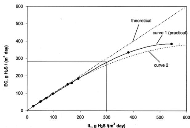
**Fig. 4.** Variation of biofilter elimination capacity (EC) versus  $\text{H}_2\text{S}$  loading rate (IL). Curve 1: Biotrickling filter packed with plastic fibres and volcanic rocks,  $0.014\text{-m}^3$  packing volume; Curve 2: Biotrickling filter packed with plastic fibres,  $0.012\text{-m}^3$  packing volume (Soreanu et al. 2007).
