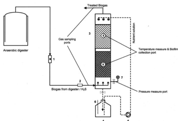
**Fig. 1.** Experimental installation set-up. 1: gas flowmeter; 2: gas equalization bottle; 3: biotrickling filter (packing bed dimension: 15-cm diameter; 0.8-m total height; 0.014-m<sup>3</sup> total volume); 4: nutrient solution tank; 5: peristaltic pump; 6: pH electrode; 7: manometer; 8: thermocouple. Open hatching: plastic fibre (0.35 m media height); shaded hatching: volcanic rocks (0.45 m media height).
