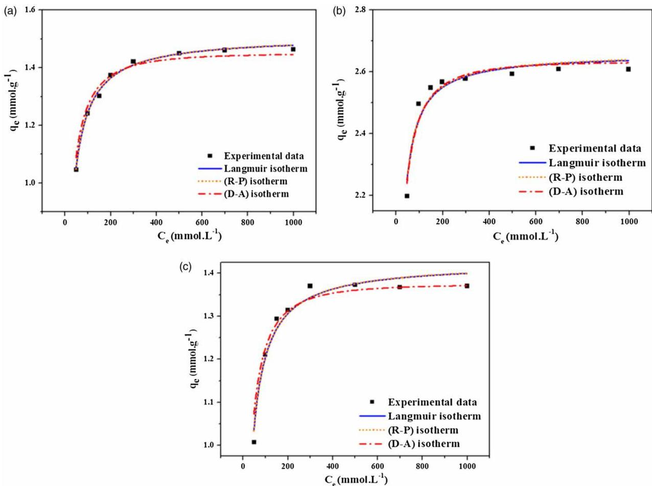
**Figure 1** | Experimental data and adsorption isotherms determined by non-linear regression of fluoride (a), nitrate (b) and sulfate (c) ions onto unmodified AFN membrane at 298 K.
