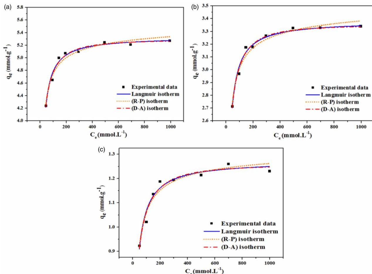
Figure 4 | Experimental data and adsorption isotherms determined by non-linear regression of fluoride (a), nitrate (b) and sulfate (c) ions onto modified AFN membrane at 298 K.
