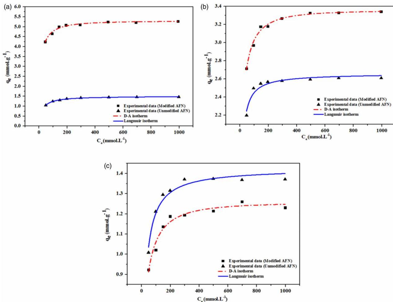
**Figure 5** | Adsorption isotherms of fluoride (a), nitrate (b) and sulfate (c) ions on the modified and the unmodified AFN membrane at 298 K.
