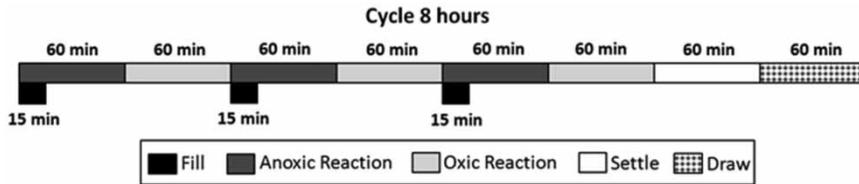
**Figure 1** | Operational scheme of SBR cycle.
