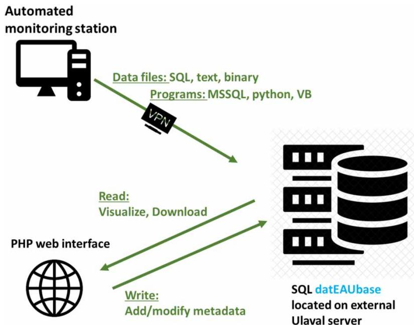
Figure 4 | Data flow design of the datEAUbase.
