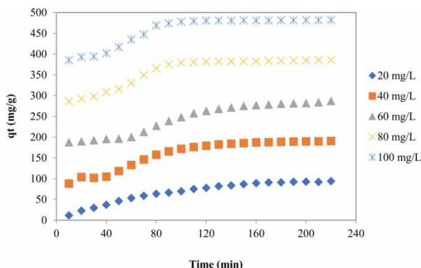
**Figure 4** | The effect of contact time on the adsorption of the CV dye onto the CWMS (adsorption conditions: pH 6; adsorbent dosage 0.2 g/L; temperature 25 °C; initial dye concentration 20–100 mg/L).
