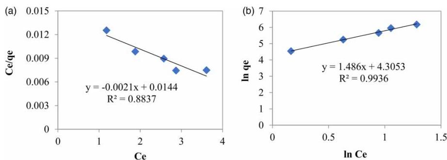
**Figure 6** | Langmuir (a) and Freundlich (b) adsorption isotherms of the CV adsorption by the CWMS with initial dye concentration in the range of 20–100 mg/L (adsorption conditions: pH 6; adsorbent dosage 0.2 g/L; temperature 25 °C; contact time 220 min).
