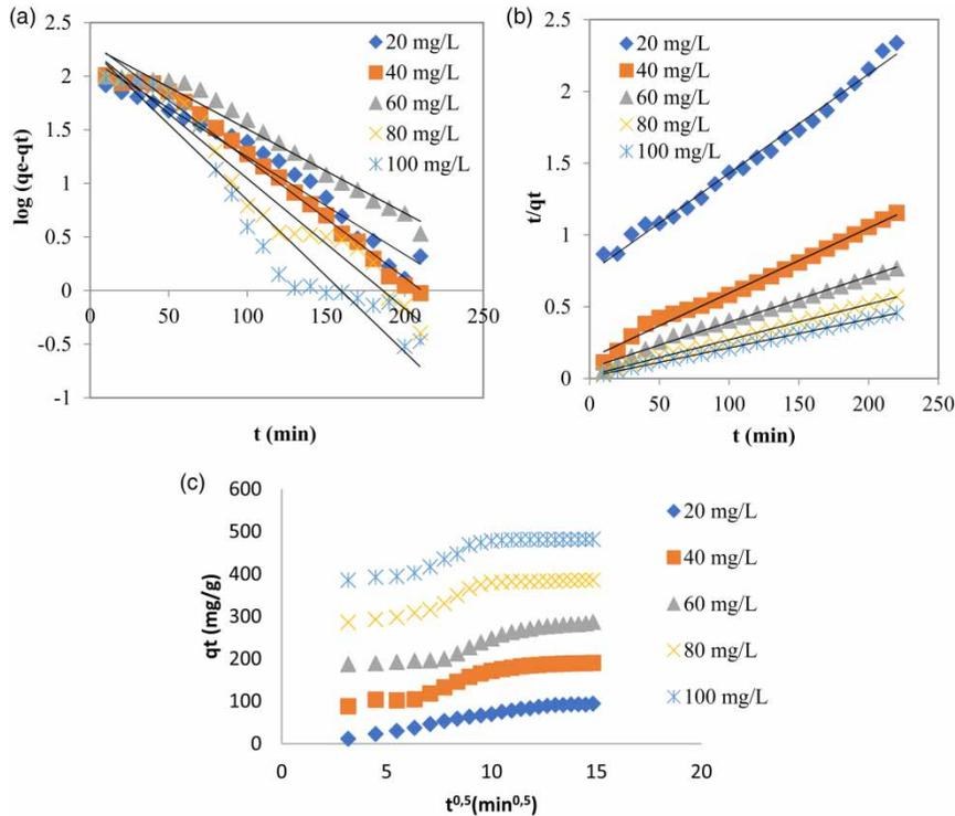
**Figure 5** | Pseudo-first order (a) pseudo-second order (b) and intraparticle diffusion model (c) plots for the CV dye adsorption onto the CWMS.
