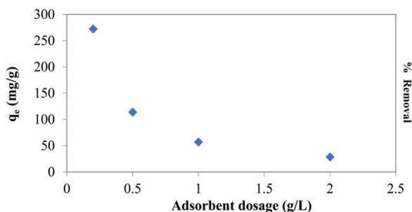
**Figure 3** | The effect of adsorbent dosage on the CV dye adsorption by the CWMS (adsorption conditions: pH 6; initial dye concentration 60 mg/L; temperature 25 °C; contact time 220 min).
