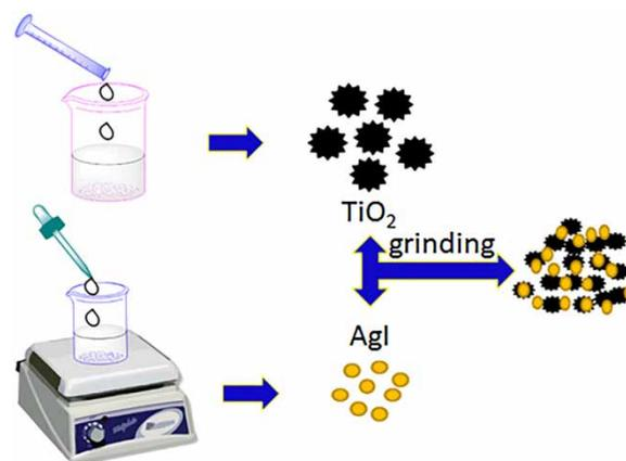
Figure 1 | Illustration of the synthetic route to AgI/TiO<sub>2</sub> composites.
