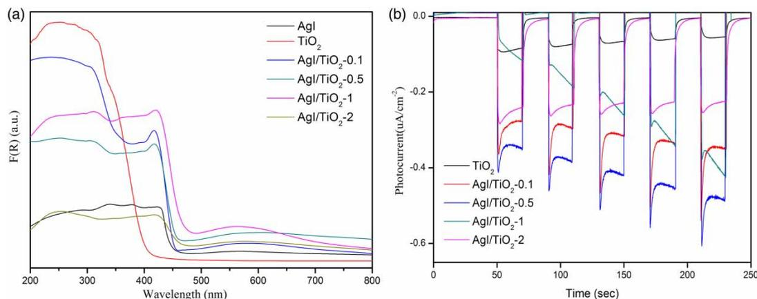
**Figure 5** | (a) UV-Vis spectra of AgI, TiO<sub>2</sub> and AgI/TiO<sub>2</sub> composites; (b) photocurrent response of TiO<sub>2</sub> and AgI/TiO<sub>2</sub> composites.
