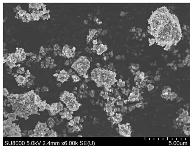
Figure 2 | SEM image of AgI/TiO<sub>2</sub>-0.5 composite.
