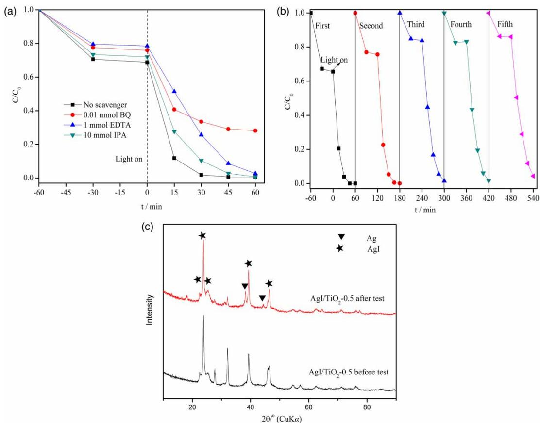
**Figure 7** | (a) Effects of different scavengers over AgI/TiO<sub>2</sub>-0.5 composite for RhB degradation; (b) reusability of AgI/TiO<sub>2</sub>-0.5 composite for RhB degradation; (c) comparison of XRD patterns of AgI/TiO<sub>2</sub>-0.5 composite before and after photocatalytic test.
