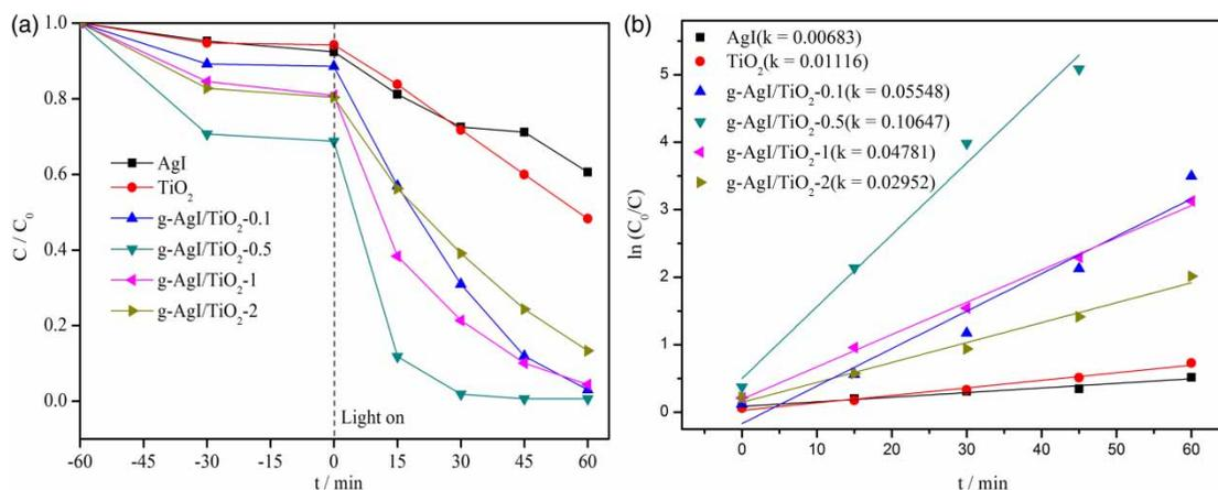
**Figure 6** | (a) Photocatalytic performance for RhB degradation over AgI, TiO<sub>2</sub> and AgI/TiO<sub>2</sub> composites under visible light irradiation; and (b) their reaction rate constants (k).
