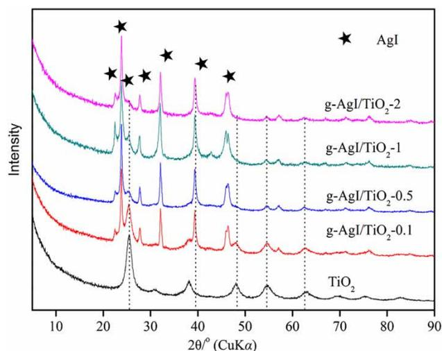
**Figure 3** | XRD patterns of TiO<sub>2</sub> and AgI/TiO<sub>2</sub> composites.
