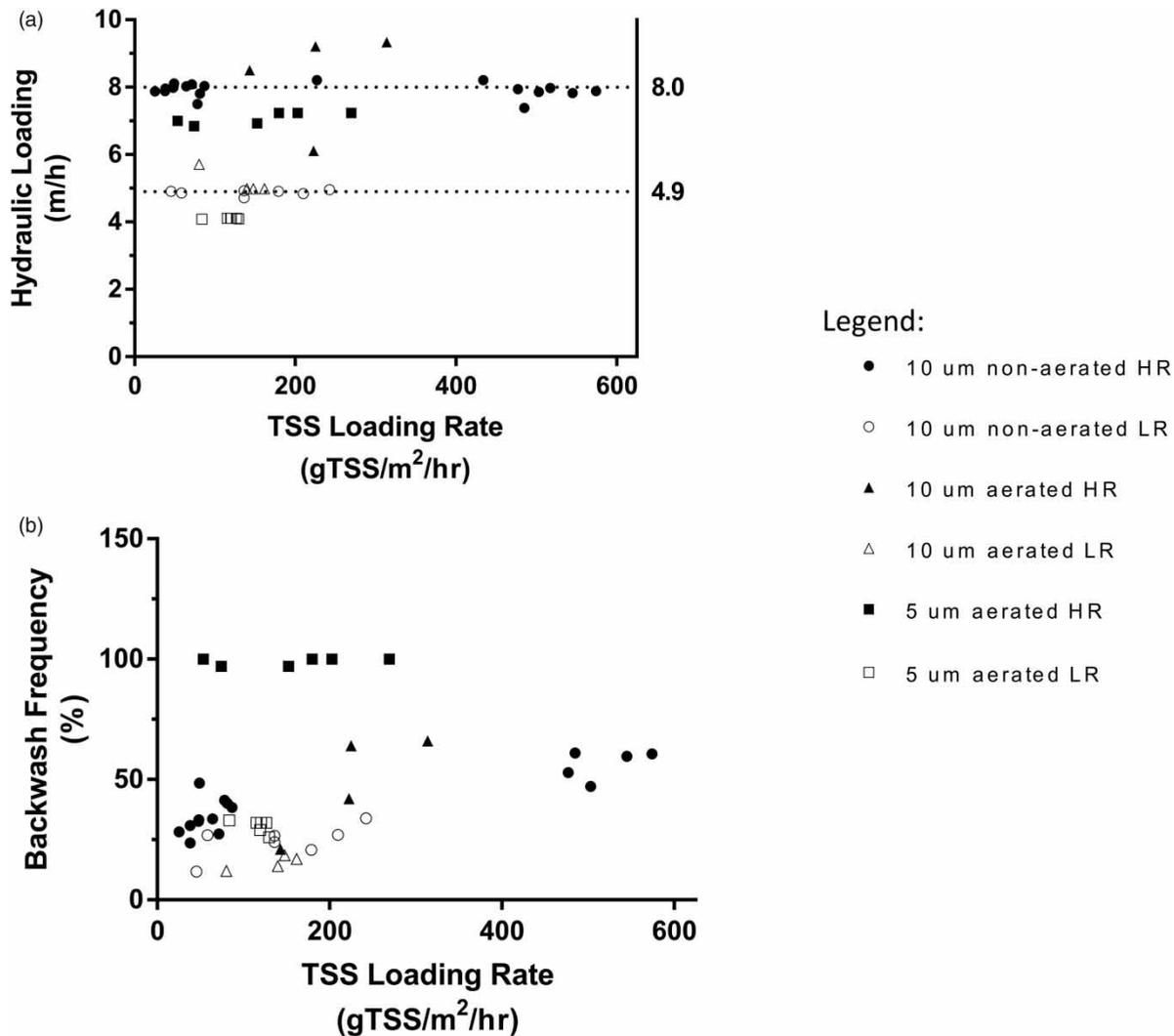
**Figure 2** | (a) Hydraulic LR across TSS LR, targeted (dotted lines) and measured (symbols) hydraulic LRs versus solids LR, and (b) backwash frequency versus solids LR.
