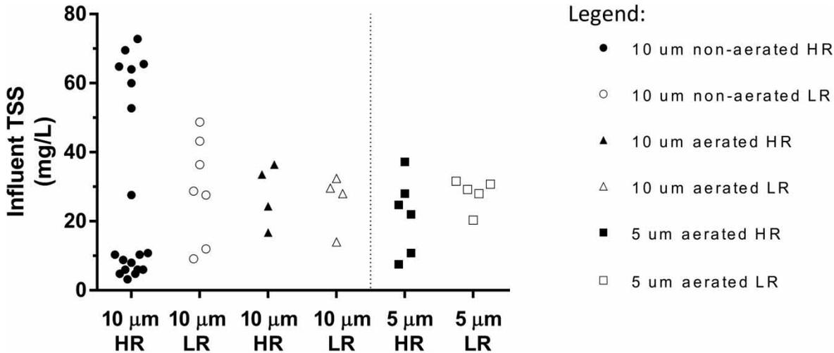
**Figure 1** | Range of influent TSS concentrations for various filter types and operational conditions across hydraulic LRs.
