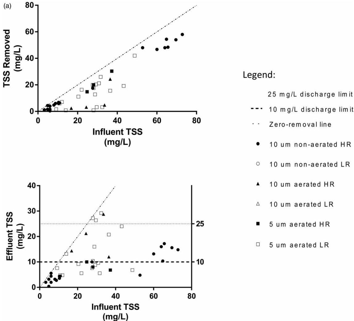
**Figure 3** | (a) TSS removal versus influent TSS concentration, TSS removed (symbols) and theoretical 100% removal (dotted line), and (b) TSS effluent (symbols) and theoretical 100% removal (dotted line), typical effluent TSS concentration limits (horizontal dashed line).
