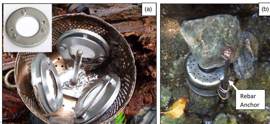
Figure 2 | (a) Photo of three POCIS disks installed within the outer protective cage with the lid removed. Close-up photo of disk provided in inset (image courtesy of Environmental Sampling Technologies). (b) Photo of POCIS deployed within a watercourse, including anchor rebar, and weighed down with large rocks to further prevent movement during high flows.
