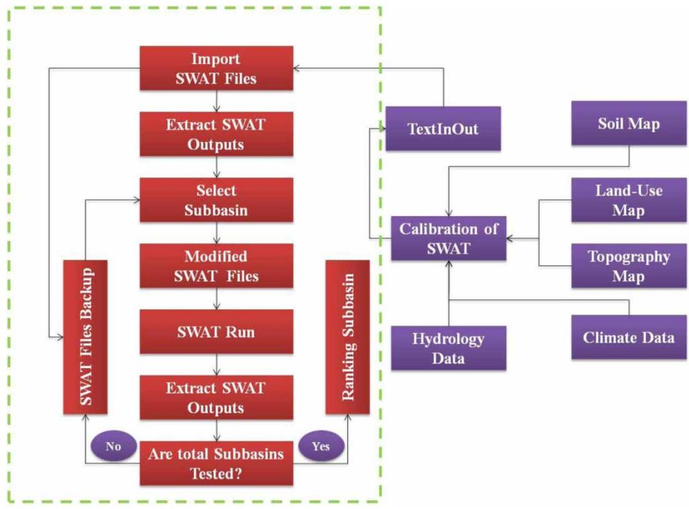
Figure 3 | Flowchart for the different processes during prioritizes of sub-watershed. The boxes within the dashed line denotes the SWAT-URA.
