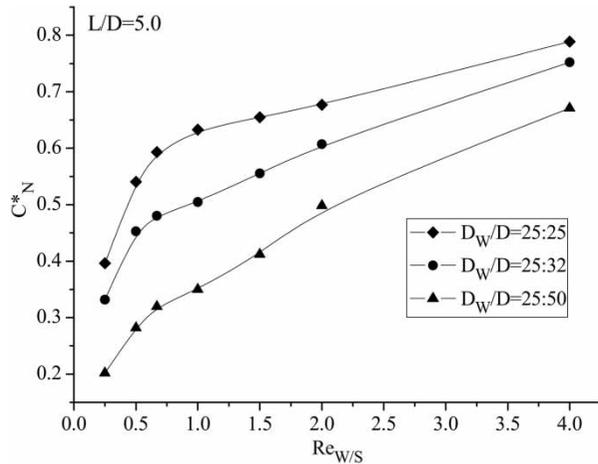
**Figure 3** | Normalized north outlet concentration with  $D_W/D = 25/25$ ,  $25/32$ , and  $25/50$  when  $Re_{W/S} = Re_{N/E}$ .
