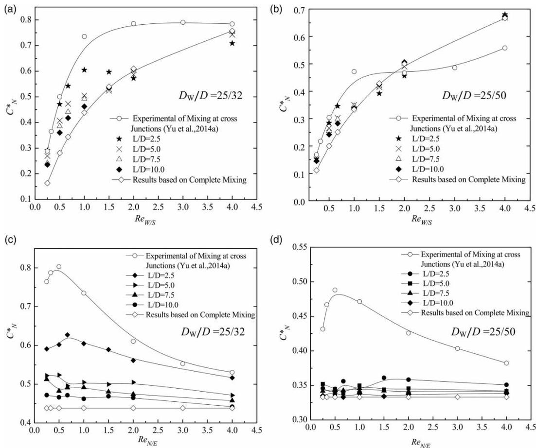
**Figure 2** | Normalized north outlet concentration with  $D_W/D = 25/32$  and  $25/50$ : (a) and (b)  $Re_{W/S} \neq 1$  and  $Re_{N/E} = 1$ ; (c) and (d)  $Re_{W/S} = 1$  and  $Re_{N/E} \neq 1$ .
