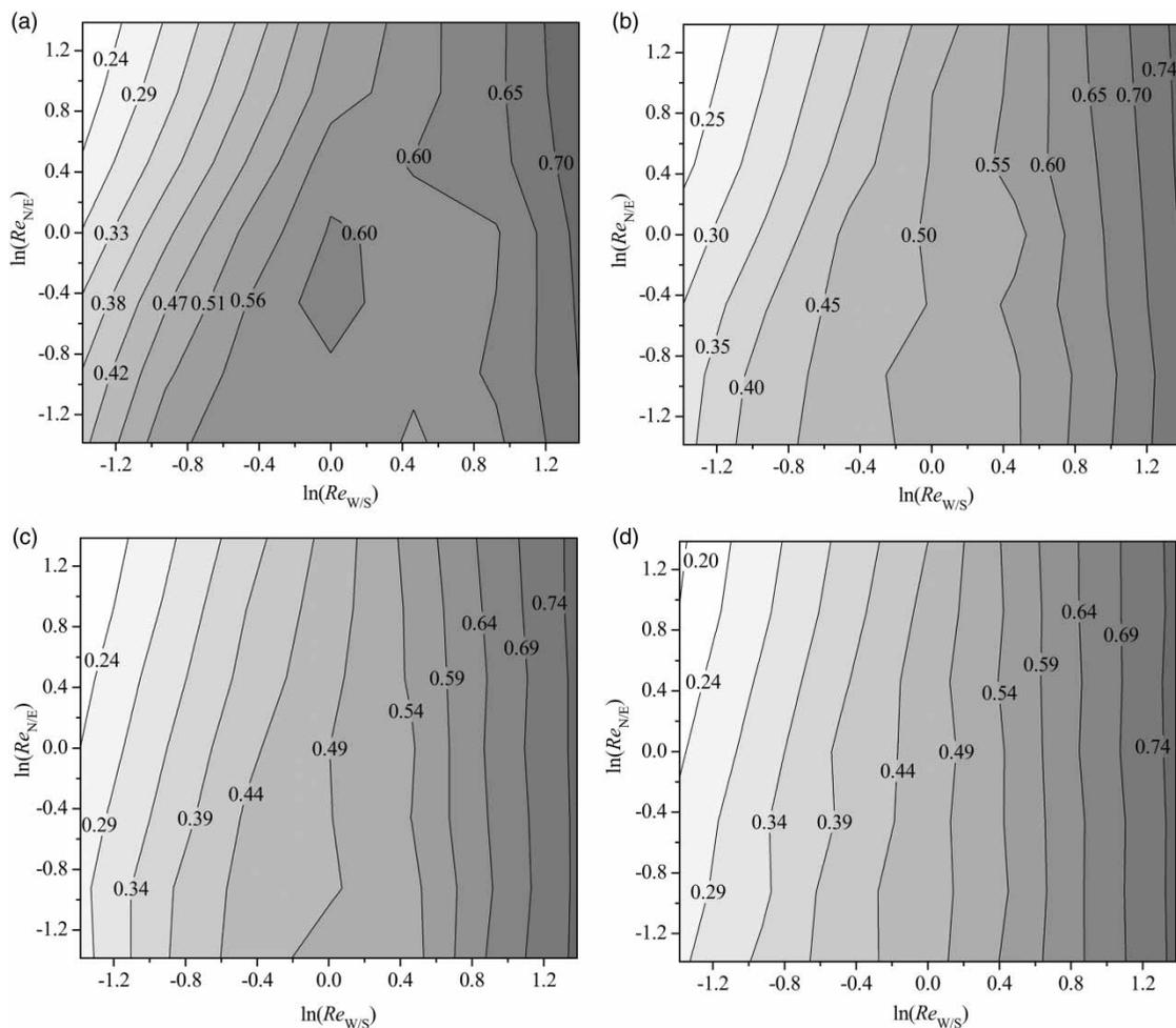
**Figure 4** | Contour graphs of  $C_N^*$  with  $D_W/D = 25/32$ : (a)  $L/D = 2.5$ ; (b)  $L/D = 5.0$ ; (c)  $L/D = 7.5$ ; and (d)  $L/D = 10.0$ .
