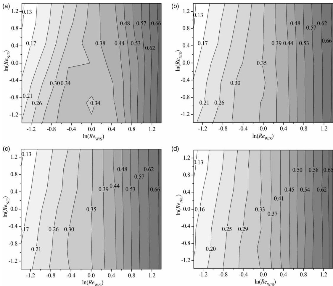
Figure 5 | Contour graphs of  $C_N^*$  with  $D_W/D = 25/50$ : (a)  $L/D = 2.5$ ; (b)  $L/D = 5.0$ ; (c)  $L/D = 7.5$ ; and (d)  $L/D = 10.0$ .
