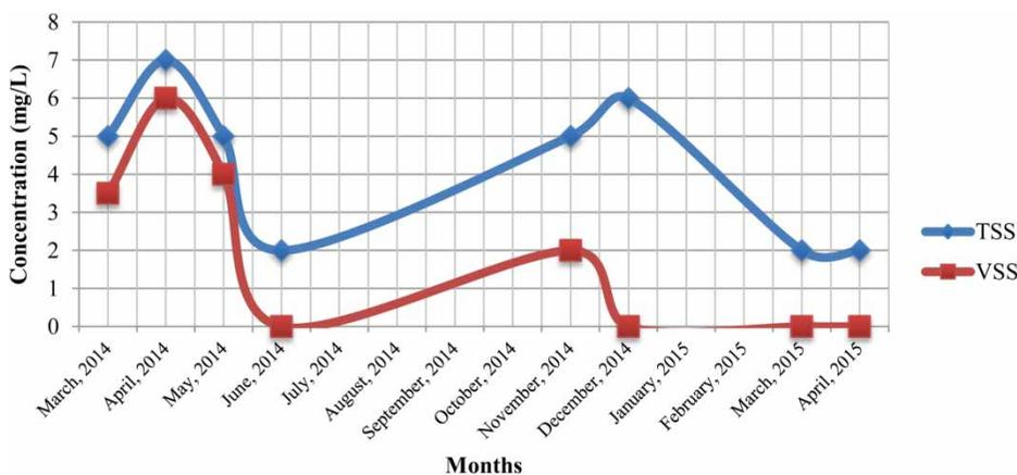
Figure 5 | Suspended solids concentration in treated grey water.
