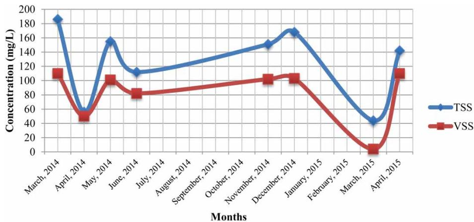
Figure 3 | Suspended solids concentrations in raw grey water.
