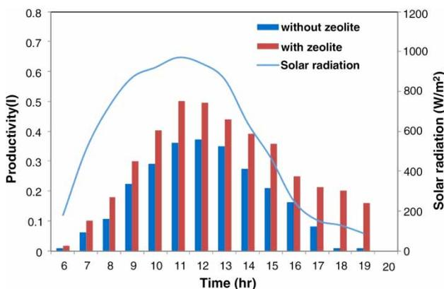
**Figure 4** | Hourly variation of freshwater production for a solar still filled with and without zeolite at  $\phi = 0.05$ .
