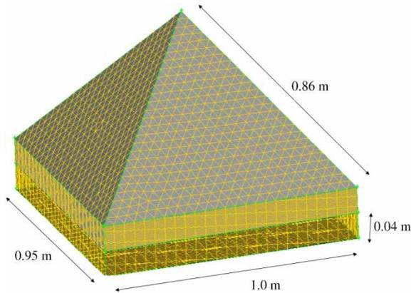
Figure 3 | Computational domain and the grid generation using Gambit.
