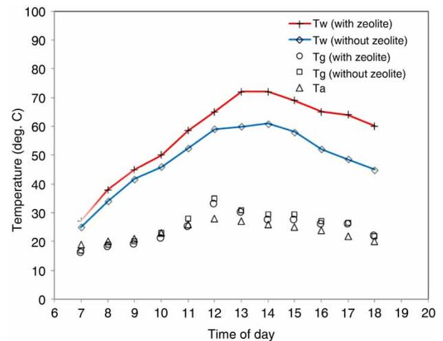
**Figure 5** | Hourly variation of basin water temperature ( $T_w$ ), glass cover temperature ( $T_g$ ), and ambient temperature ( $T_a$ ) during one day at  $\phi = 0.05$ .
