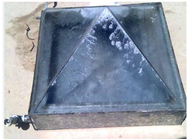
Figure 1 | Photograph of pyramid-shaped solar still.
