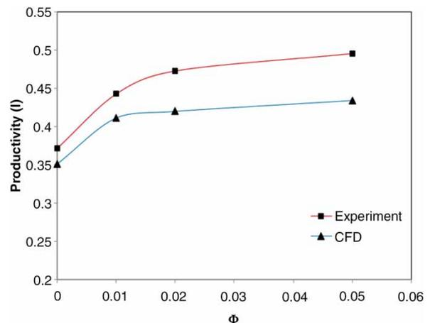
**Figure 6** | Comparison of experimental and CFD simulation of productivity of solar still as a function of zeolite volume fraction at time 13.00 h.
