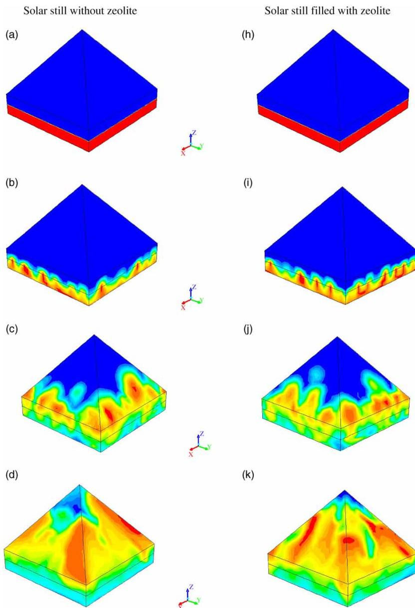
**Figure 7** | Contours of water vapor fraction for still with (figure from (h) to (n)) and without (figure from (a) to (g)) zeolite particle load, ( $\phi = 0.05$ ), time 13.00 h. (Continued.)
