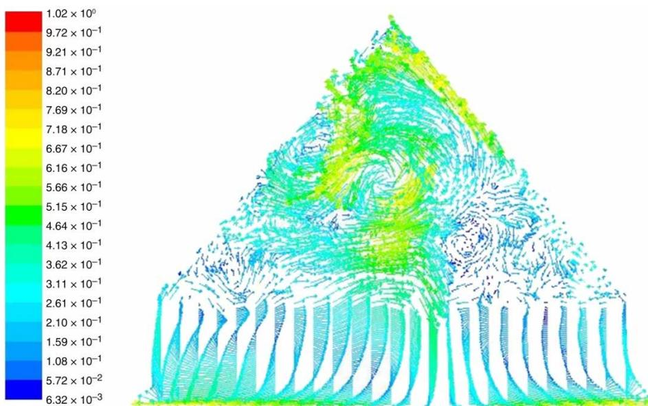
Figure 8 | Velocity vectors in the middle of the solar still without zeolite particles.
