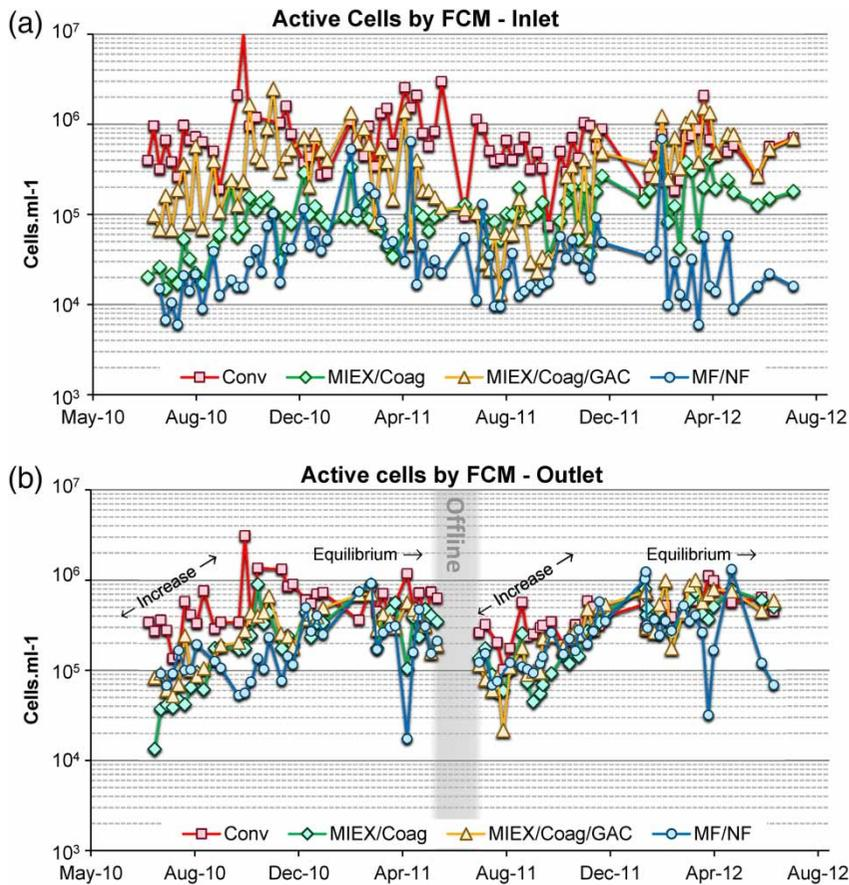
**Figure 4** | Comparison of active (membrane intact) cells by FCM of bulk water at (a) inlet and (b) outlet of PDS following 78 hour detention. Offline period represents an unplanned maintenance event during which the PDS were quiescent.
