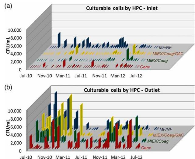
**Figure 3** | HPC in the bulk water prior to entry and after detention within the PDS. (a) Inlet; (b) outlet.
