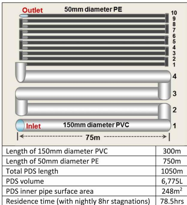
Figure 1 | PDS layout schematic and technical specifications.
