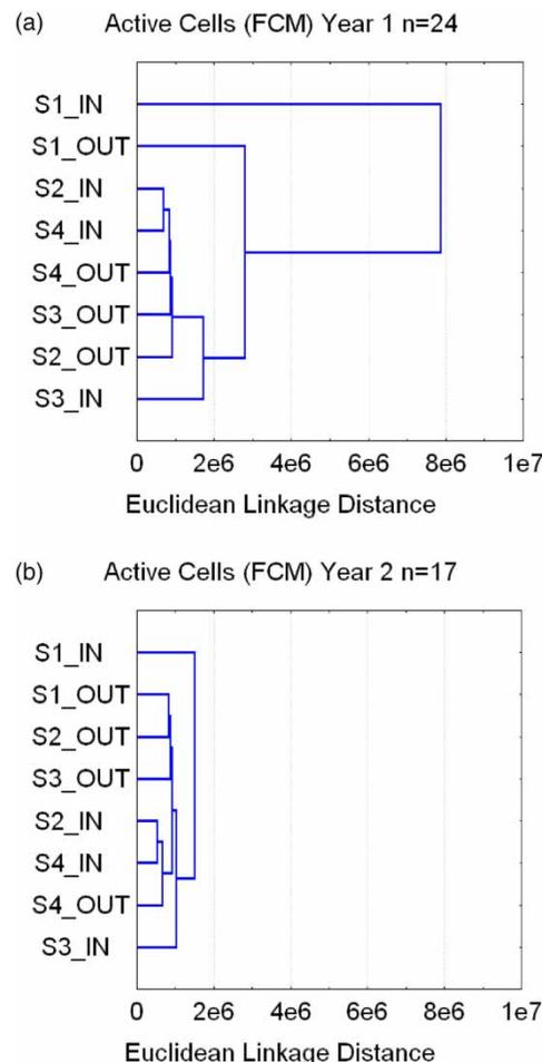
**Figure 6** | Dendrogram for relationship of PDS inlets and outlets by FCM active cell counts in: (a) Year 1 (July 2010–June 2011) and (b) Year 2 (August 2011–July 2012). S1 = Conv; S2 = MIEX/Coag; S3 = MIEX/Coag/GAC; S4 = MF/NF.
