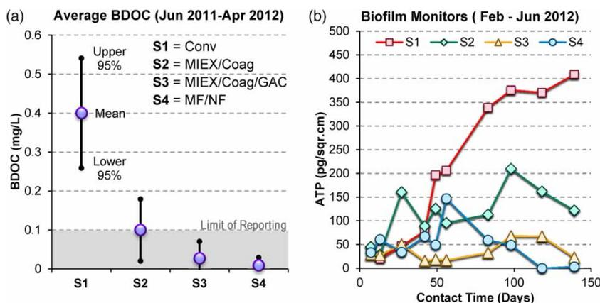
**Figure 7** | Biological growth potential measures for PDS inlet water: (a) average BDOC and (b) biofilm monitor activity by ATP.
