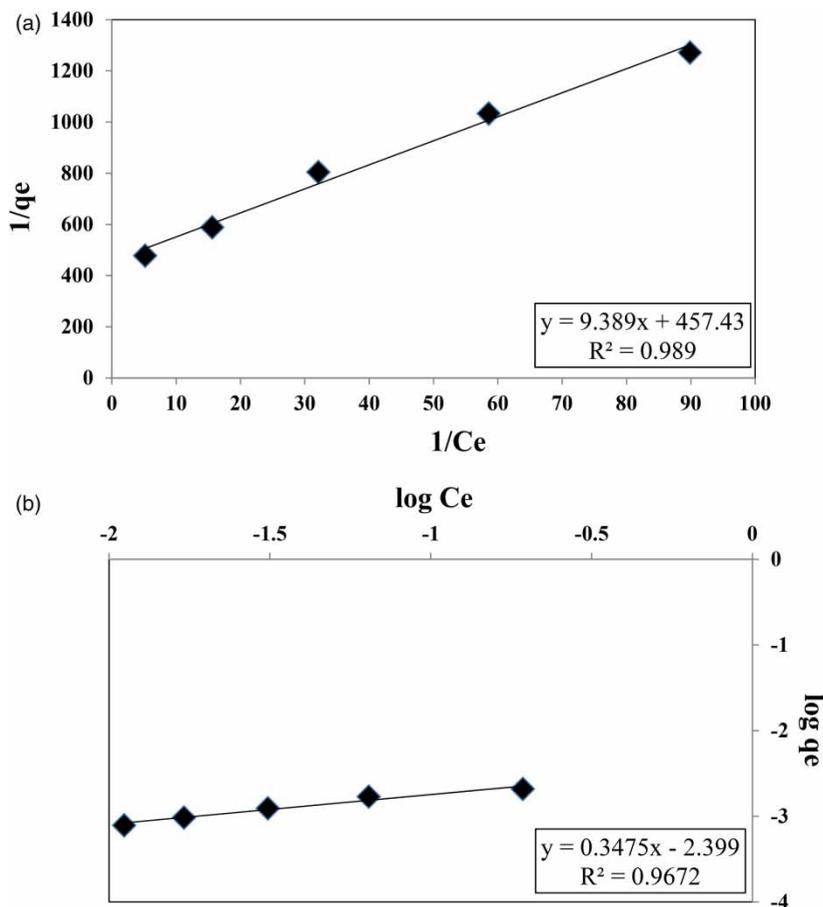
**Figure 12** | Isotherm plots for As(III) adsorption on ICZ. (a) Langmuir isotherm. (b) Freundlich isotherm ( $\text{pH} = 7$ , initial concentration = 400  $\mu\text{g/L}$ , temperature = 40  $^\circ\text{C}$ , contact time = 30 min and mixing intensity = 500 rpm).
