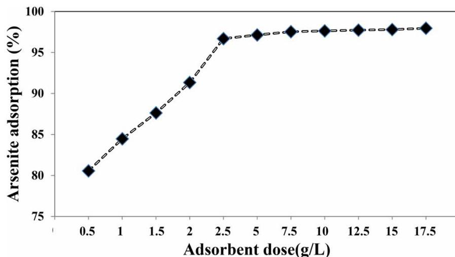
**Figure 10** | Effect of adsorbent dose on arsenite adsorption using ICZ (pH = 7, temperature = 25 °C, initial concentration = 400 µg/L, contact time = 60 min and mixing intensity = 500 rpm).
