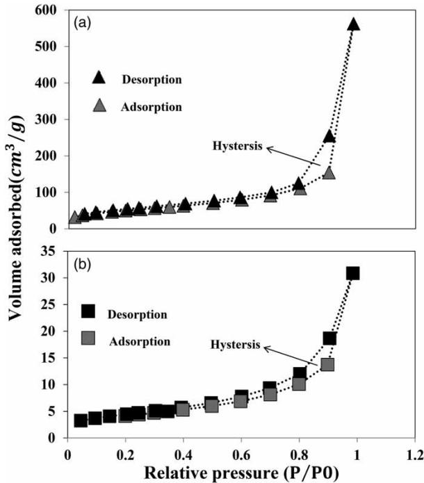
**Figure 8** |  $N_2$  adsorption–desorption isotherms of the samples at 77.3K. (a) ZSM-5 zeolite support. (b) ICZ.
