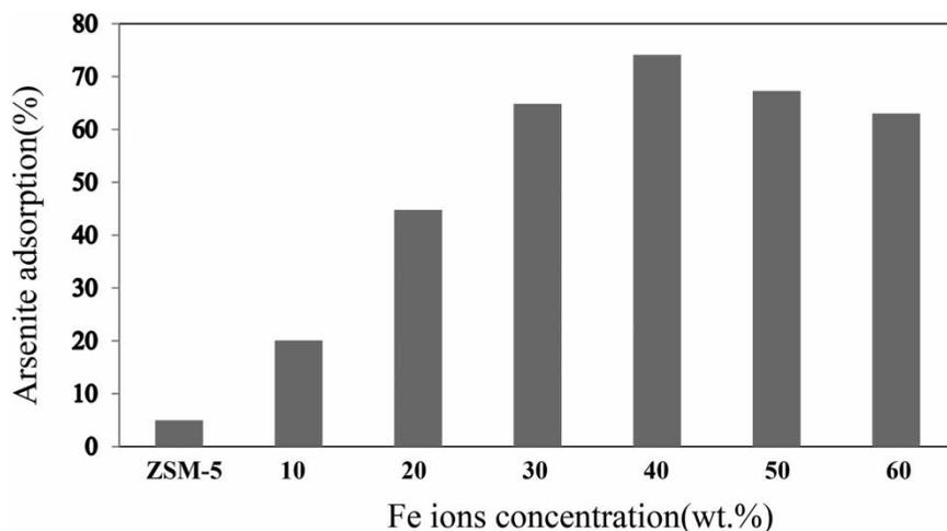
**Figure 1** | Influence of Fe loading concentration on arsenite adsorption by ICZ (calcination temperature = 400 °C, calcination time = 3 h, synthesis temperature = 30 °C and mixing intensity = 60 rpm).
