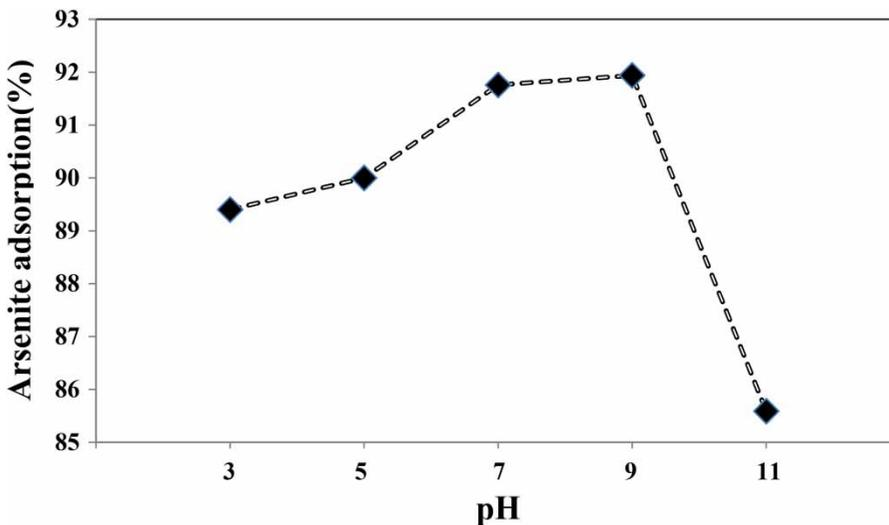
**Figure 9** | Effect the change of pH on arsenite adsorption using ICZ (adsorbent dose = 10 g/L, temperature = 25 °C, initial concentration = 400  $\mu\text{g/L}$ , contact time = 60 min and mixing intensity = 500 rpm).
