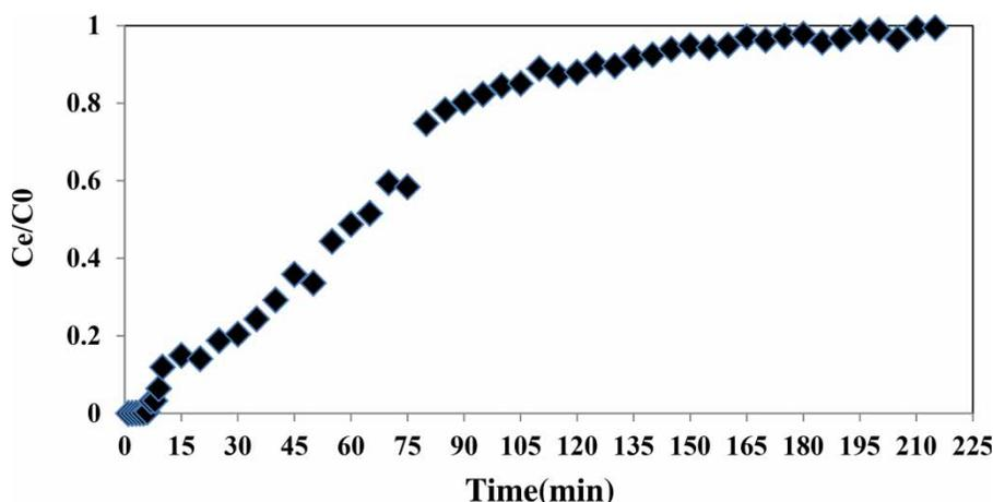
**Figure 14** | Breakthrough curve in ICZ for As(III) adsorption (initial concentration = 400  $\mu\text{g/L}$ , temperature = 40  $^{\circ}\text{C}$  volume of solution = 1 L and flow rate = 279  $\text{mL.h}^{-1}$ ).
