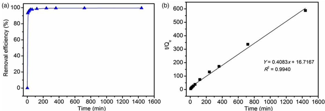
**Figure 5** | (a) Relationship between the removal efficiency and adsorption time; (b) the kinetic process fitted with a pseudo-second-order model.
