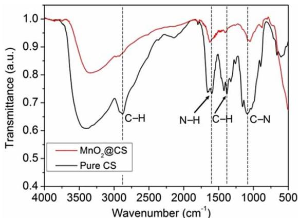
**Figure 3** | FTIR spectra of the CS NP-modified MnO<sub>2</sub> nanoflakes and the pure CS.
