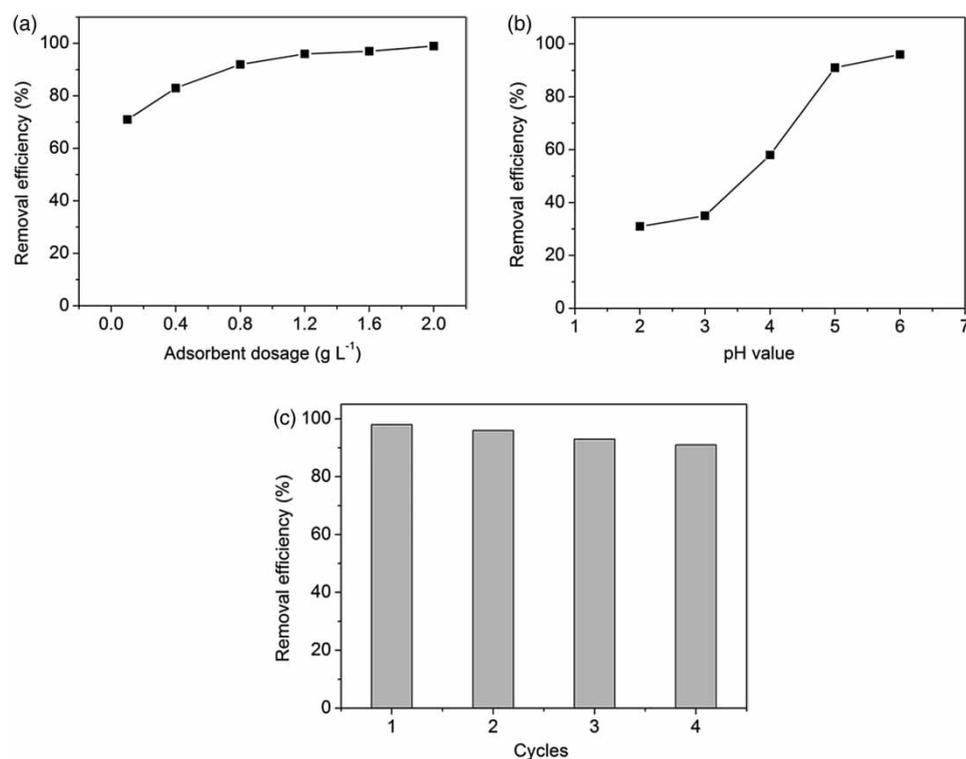
**Figure 7** | The effects of (a) adsorbent dosage and (b) pH value on Pb(II) adsorption onto the CS NP-modified MnO<sub>2</sub> nanoflakes. (c) Adsorbent regeneration cycles (conditions: initial concentration of Pb(II): 20 mg L<sup>-1</sup>; adsorbent dosage: 1 g L<sup>-1</sup>; adsorption time: 3 h; desorption time: 3 h; 0.05 mol L<sup>-1</sup> EDTA as regeneration agent).
