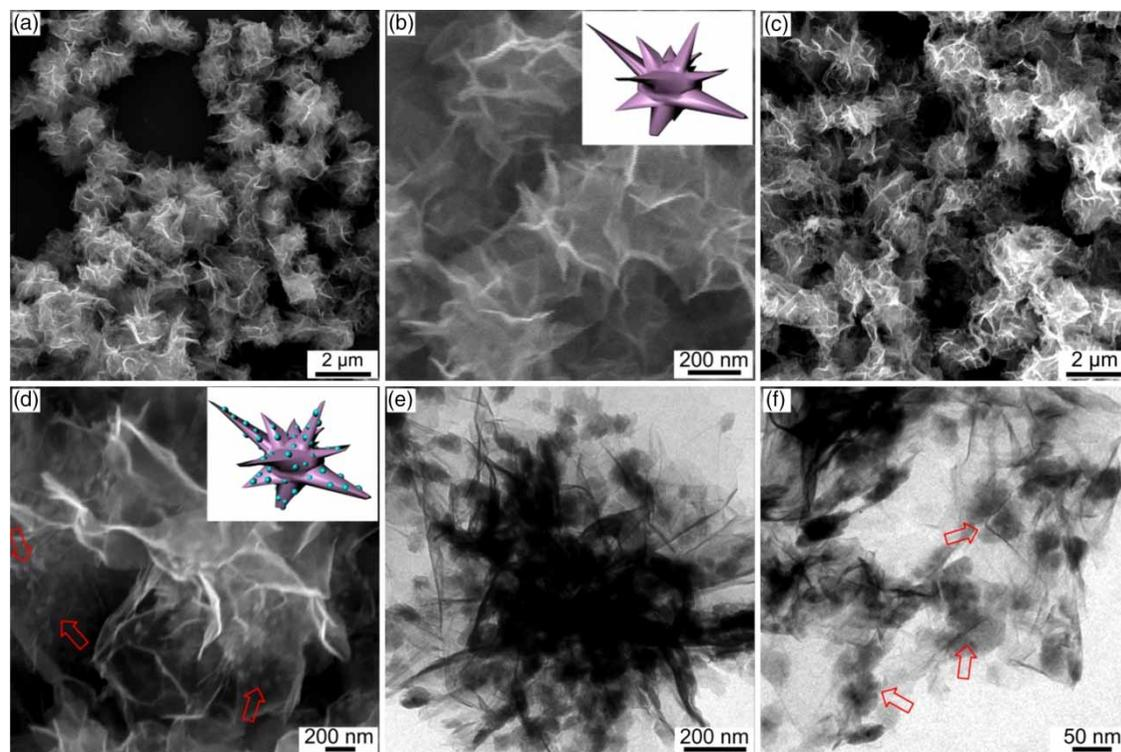
**Figure 1** | (a) Low- and (b) high-magnification FESEM images of the MnO<sub>2</sub> nanoflakes; (c), (d) FESEM images and (e), (f) TEM images of the MnO<sub>2</sub> nanoflakes modified with CS NPs. Insets in (b) and (d) are corresponding schematic illustrations of nanoflakes without and with NP modifications, respectively.
