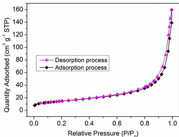
**Figure 4** | Typical N<sub>2</sub> adsorption–desorption isotherm of the CS NPs-modified MnO<sub>2</sub> nanoflakes.
