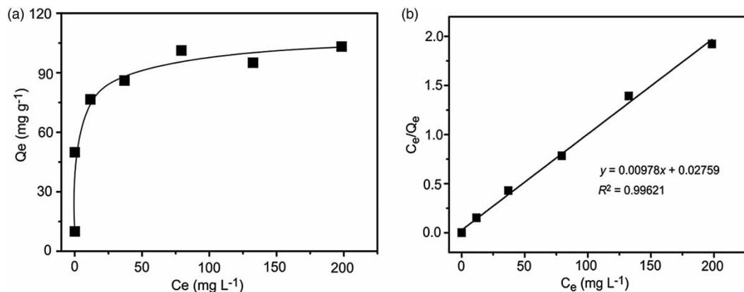
**Figure 6** | (a) The saturated adsorption isotherm of the CS NP-modified MnO<sub>2</sub> nanoflakes; (b) the fitting result by a Langmuir isotherm model.
