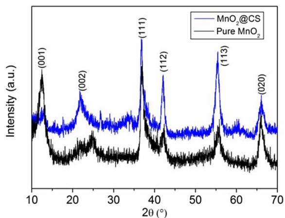
**Figure 2** | XRD patterns of the MnO<sub>2</sub> nanoflakes before and after modification with CS NPs.
