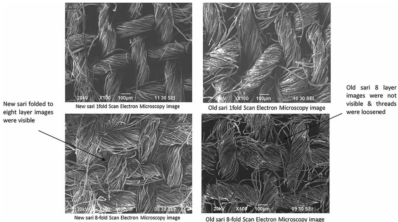
Figure 3 | Comparison of electron micrographs of one- and eight-layer new and old cotton sari.
