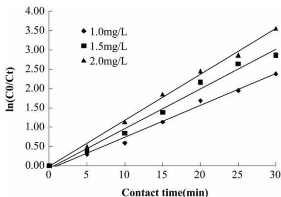
Figure 6 | First-order kinetic plot for the decay of  $\text{ClO}_2$ .
