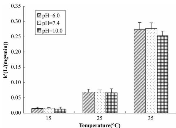
**Figure 8** | Effect of temperature and pH on PAE inactivation rate constant.
