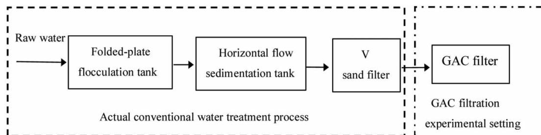
Figure 1 | Schematic diagram of the conventional treatment process and GAC filter.
