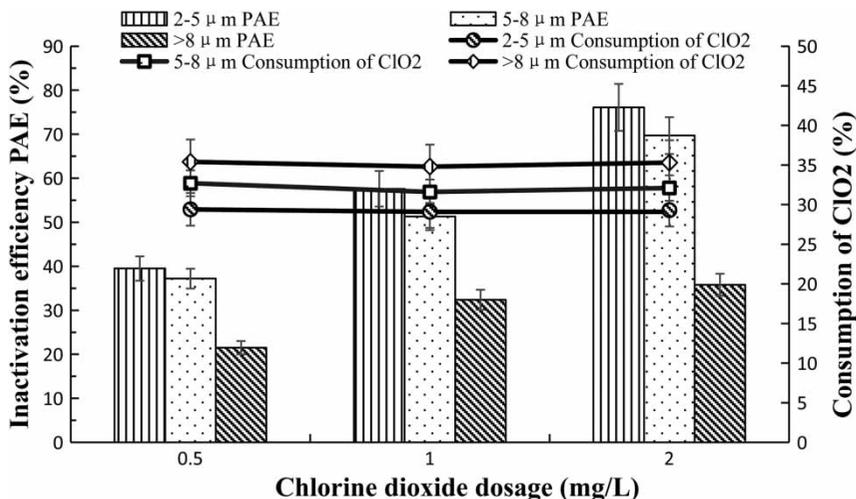
Figure 5 | Influence of particle distribution on PAE inactivation rate at ambient temperature with particle concentration of  $2 \times 10^3$  counts/mL for 30 min.
