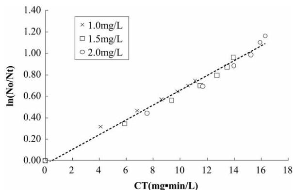
Figure 7 | Inactivation kinetics of PAE with  $\text{ClO}_2$  at pH 7.4 and 25 °C.
