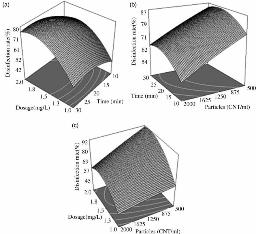
**Figure 4** | Response surface plots for PAB inactivation as an interaction function of independent variables (temperature: 25 °C; pH: 7.4). (a) Particle concentration: approximately 1,250 counts/mL; (b) ClO<sub>2</sub> dosage: 1.5 mg/L; (c) exposure time: 20 min.
