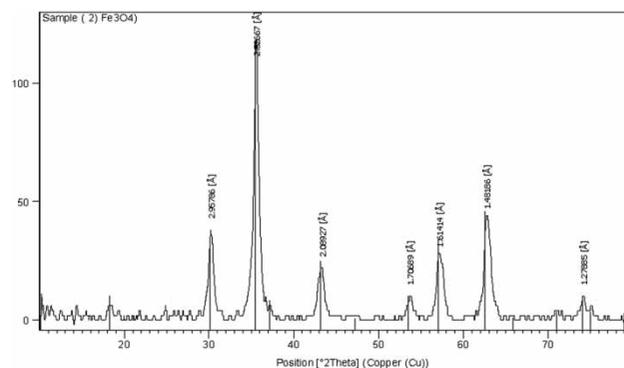
Figure 2 | XRD of bare  $\text{Fe}_3\text{O}_4$  NPs.
