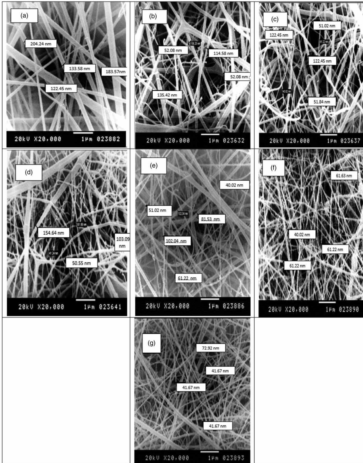
Figure 3 | SEM images of CA/Fe<sub>3</sub>O<sub>4</sub> (0, 0.2, 0.5, 1.0, 1.5, 2.0 and 2.5 wt/v) composite NFs: (a)–(g) respectively.
