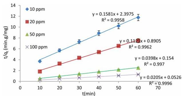
Figure 11 | PSO plot of Pb(II) adsorption on 0.1 g CA/Fe<sub>3</sub>O<sub>4</sub> NFs (2.5% wt/v) in 50 ml solution at pH = 6 and 27 °C.
