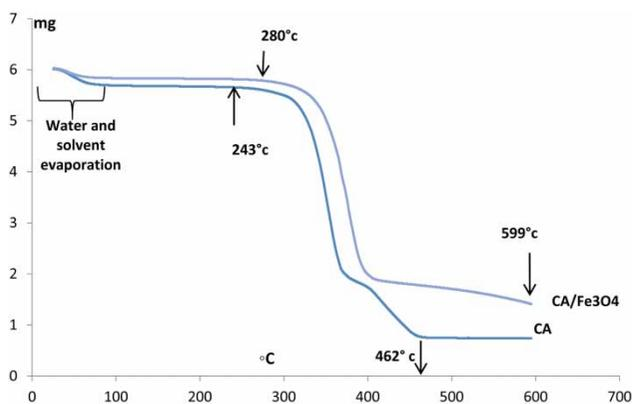
**Figure 4** | Thermograms of CA NFs (a) and CA/Fe<sub>3</sub>O<sub>4</sub> (2.5% wt/v) NFs (b).
