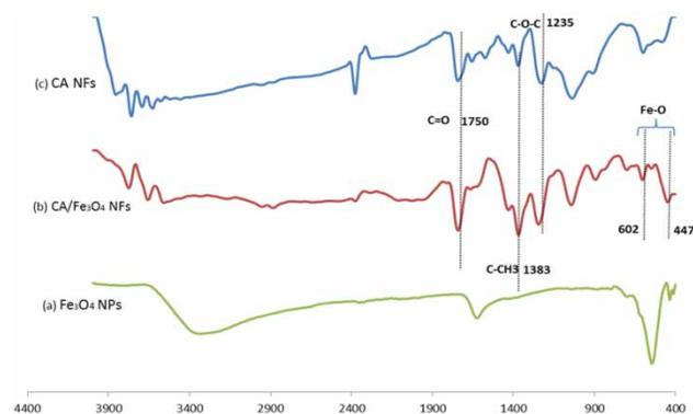
**Figure 5** | FT-IR spectrum of Fe<sub>3</sub>O<sub>4</sub> NPs (a), CA/Fe<sub>3</sub>O<sub>4</sub> (2.5% wt/v) nanocomposite fibers (b) and CA nanofibers (c).
