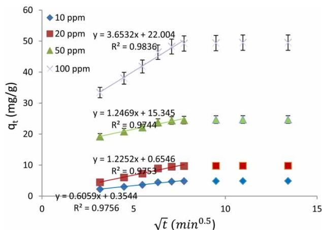
Figure 12 | Intra-particle diffusion plot of Pb(II) adsorption on 0.1 g CA/Fe<sub>3</sub>O<sub>4</sub> NFs (2.5% wt/v) in 50 ml solution at pH = 6 and 27 °C.
