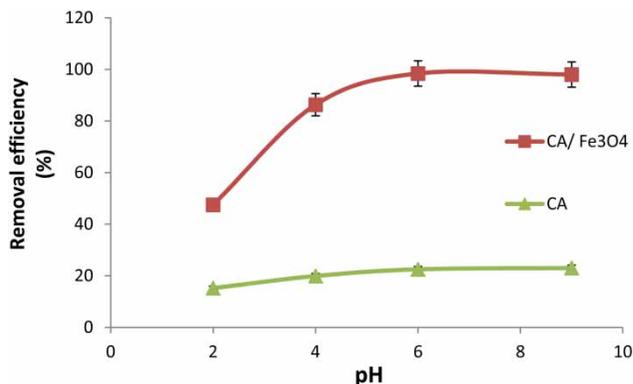
**Figure 9** | Effect of pH on Pb(II) removal efficiency by the CA nanofibers and the CA/Fe<sub>3</sub>O<sub>4</sub> composite nanofibers. Reaction conditions: initial metal ion concentration 50 mg/L; adsorbent amount 0.1 g/50 ml; adsorption time 24 h; and temperature 27 °C.
