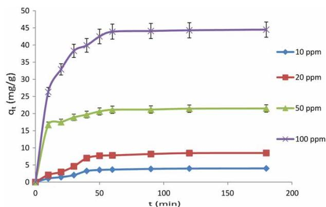
Figure 7 | Adsorption of Pb(II) on 0.1 g CA/ $\text{Fe}_3\text{O}_4$  NFs (2.5% wt/v) in 50 ml solution with different initial concentrations at pH = 6 and  $27\text{ }^\circ\text{C}$ .
