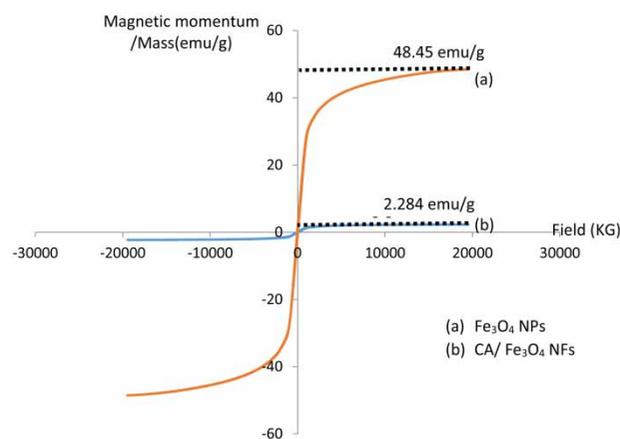
Figure 6 | VSM graphs of  $\text{Fe}_3\text{O}_4$  NPs (a) and CA/ $\text{Fe}_3\text{O}_4$  NFs (2.5% wt/v) (b).
