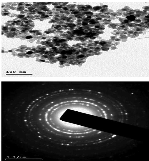
Figure 1 | TEM micrograph and diffraction pattern of  $\text{Fe}_3\text{O}_4$  NPs.
