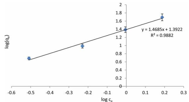
Figure 14 | Freundlich isotherm for the adsorption of Pb(II) on the CA/Fe<sub>3</sub>O<sub>4</sub> (2.5% wt/v) NFS.
