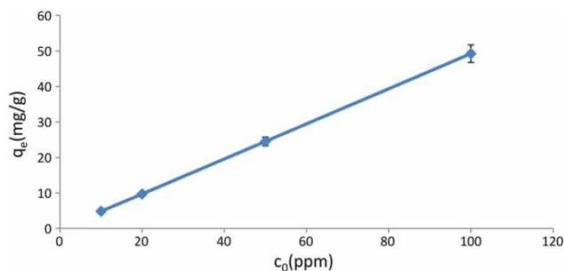
Figure 8 | The dependence of the equilibrium adsorption capacity of Pb(II) ions on the initial concentrations.
