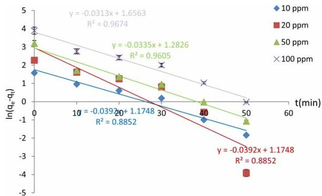
Figure 10 | PFO plot of Pb(II) adsorption on 0.1 g CA/Fe<sub>3</sub>O<sub>4</sub> NFs (2.5% wt/v) in 50 ml solution at pH = 6 and 27 °C.
