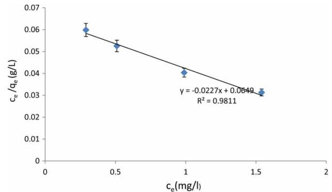
Figure 13 | Langmuir isotherm for the adsorption of Pb(II) on the CA/Fe<sub>3</sub>O<sub>4</sub> (2.5% wt/v) NFS.
