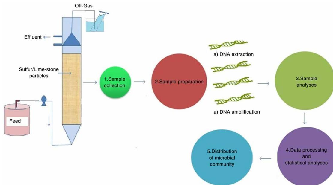
**Figure 1** | Scheme showing the application of 454-pyrosequencing analysis to the study of bacterial communities associated with denitrification.
