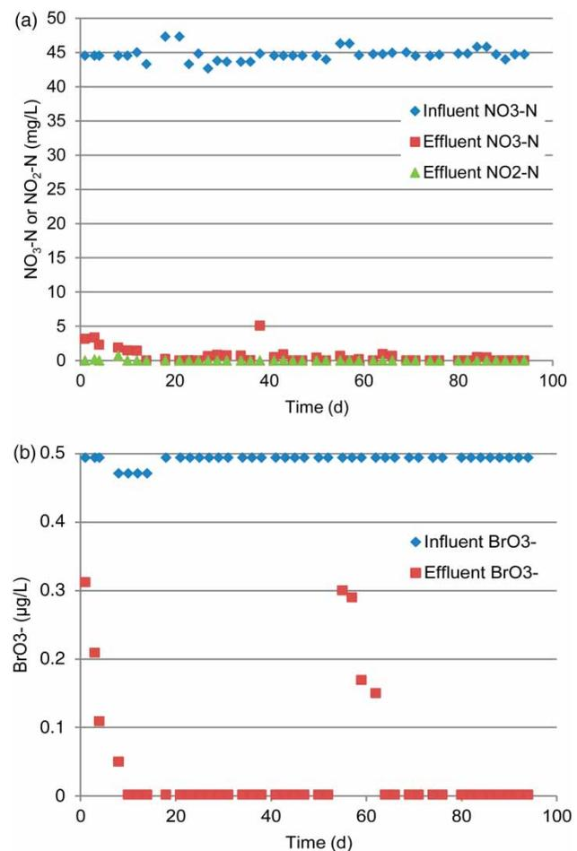
Figure 2 | Influent and effluent (a)  $\text{NO}_3\text{-N}$  or  $\text{NO}_2\text{-N}$ , and (b)  $\text{BrO}_3^-$  variations.
