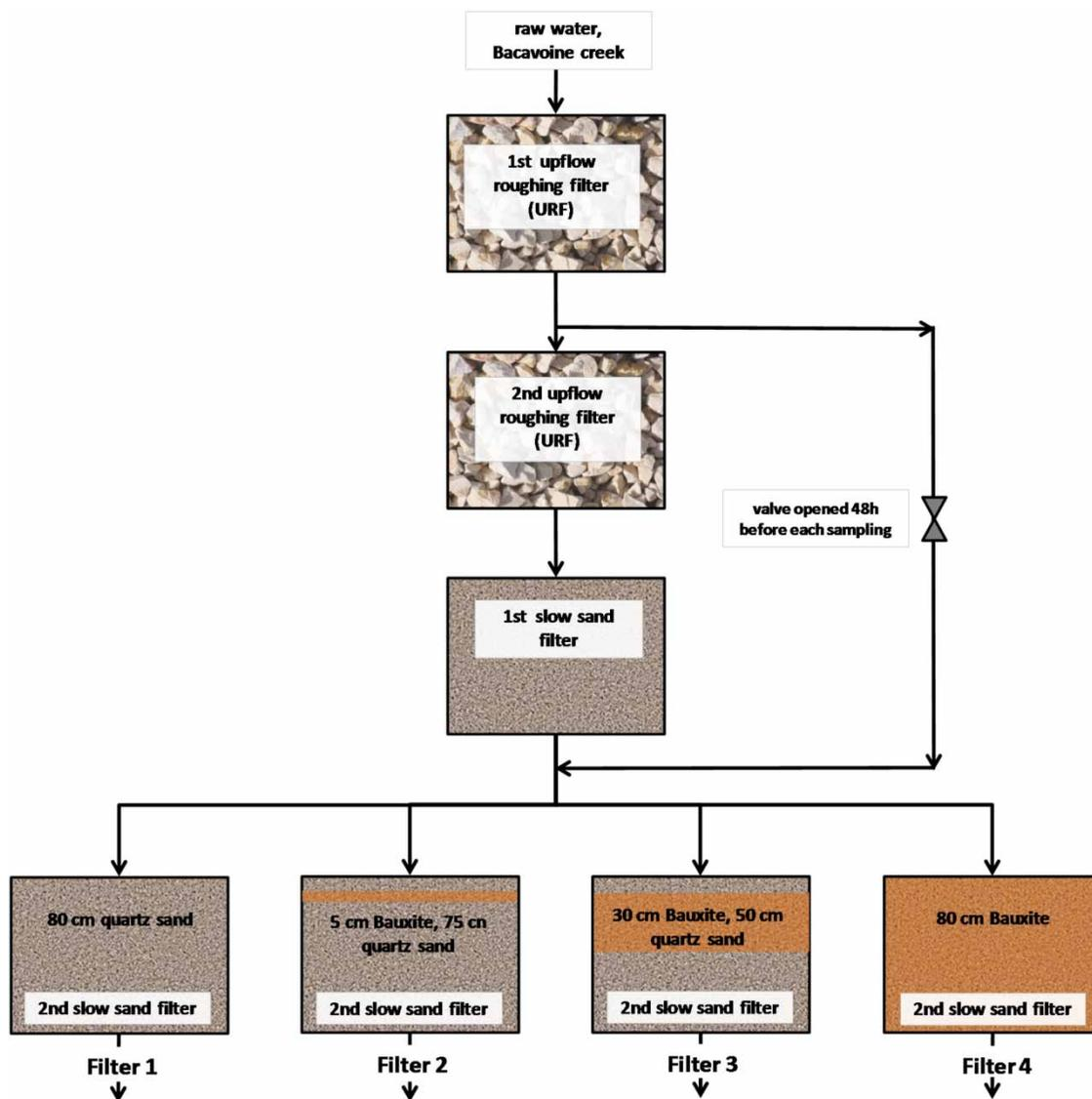
**Figure 1** | Layout of the MSF pilot plant.
