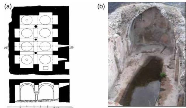
**Figure 6** | Byzantine-era cisterns at (a) Osios Loukas monastery in Boeotia, Hellas (Orlandos 1926) covered with a lowered dome (notice the intake spout) and (b) the Goulas of the castle at Leontari Arkadias (G. Antoniou).
