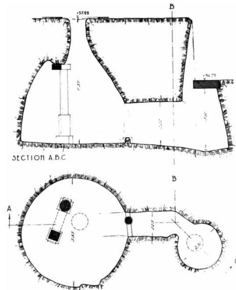
Figure 3 | Two-chambered cistern in Hellenistic Athens (Rotroff 1983).
