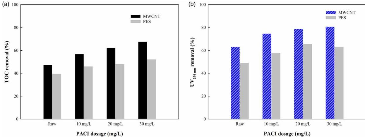
**Figure 3** | Comparison of organic matter removal of the MWCNT and PES-UF membranes with PACI flocculation: (a) TOC removal rate (%) and (b) HA (UV<sub>254 nm</sub>) removal rate (%).
