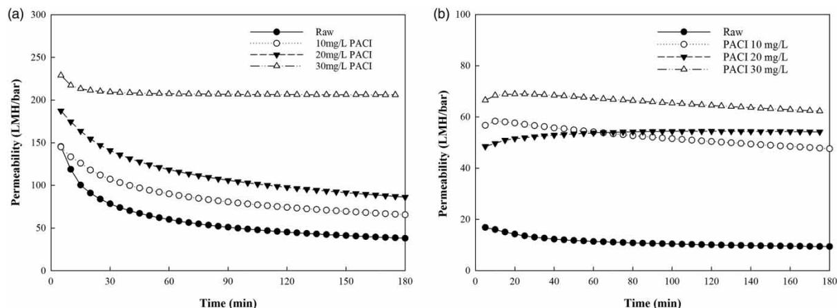
**Figure 2** | Comparison of flux behaviour between (a) MWCNT membrane and (b) PES-UF membrane with PACI flocculation.
