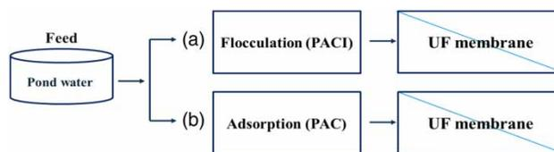
**Figure 1** | Schematic of UF coupled with (a) flocculation (PACI) and (b) adsorption (PAC) systems.
