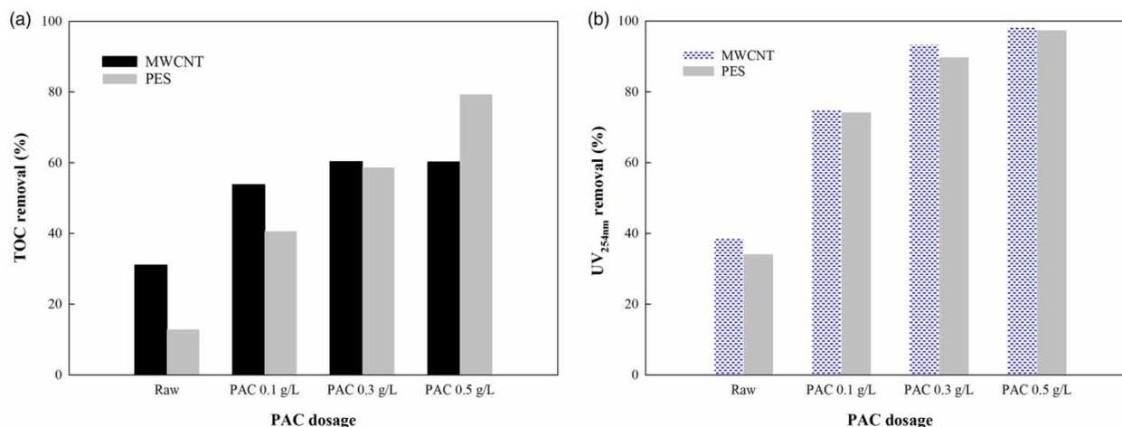
Figure 5 | Comparison of organic matter removal of the MWCNT and PES-UF membranes with PAC adsorption: (a) TOC removal rate (%) and (b) HA ( $UV_{254\text{ nm}}$ ) removal rate (%).
