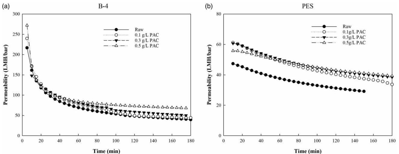
**Figure 4** | Comparison of flux behaviour between (a) MWCNT membrane and (b) PES-UF membranes with PAC adsorption.
