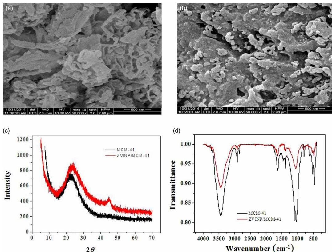
**Figure 1** | Characterization of MCM-41 and ZVINP/MCM-41: (a) scanning electron microscopy of MCM-41; (b) scanning electron microscopy of ZVINP/MCM-41; (c) XRD diffraction pattern of MCM-41 (black line) and ZVINP/MCM-41 (red line); (d) FTIR of MCM-41 (black line) and ZVINP/MCM-41 (red line). Please refer to the online version of this paper to see this figure in colour: <http://dx.doi.org/10.2166/ws.2017.003>.
