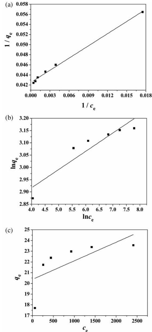
Figure 4 | (a) Langmuir, (b) Freundlich, and (c) Henry adsorption isotherm fits of NDMA removal on ZVINP/MCM-41.
