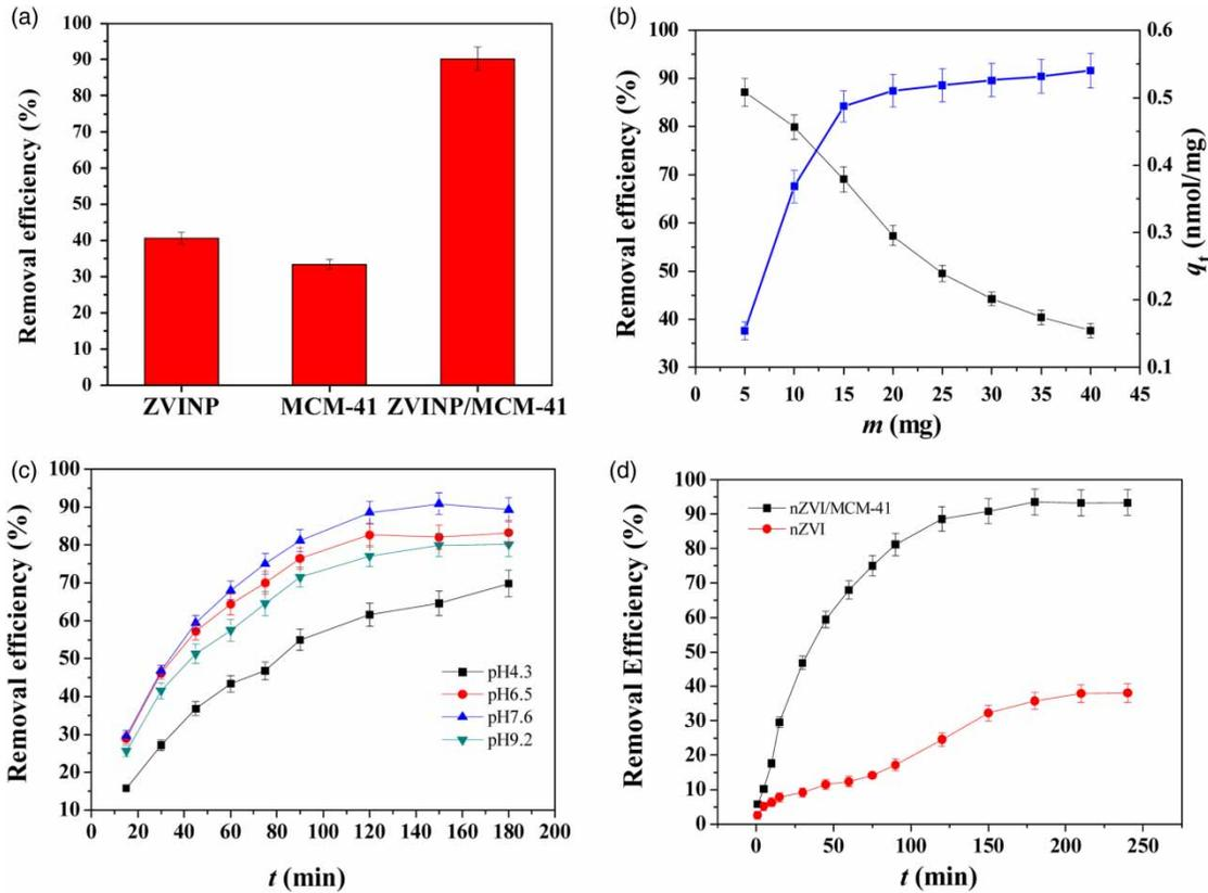
**Figure 2** | Removal efficiencies of materials: (a) ZVINP, MCM-41, and ZVINP/MCM-41; (b) ZVINP/MCM-41 dose (5 to 40 mg); (c) initial pH (4.3 to 9.2); (d) and performing time (15–240 min). (All experiments under the conditions of 1,000 mL 1.0  $\mu\text{g/L}$  NDMA solution at 25 °C.)
