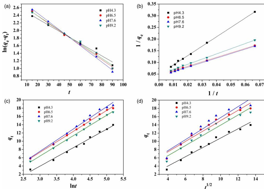
**Figure 3** | (a) First-order kinetics, (b) second-order kinetics, (c) Elovich model and (d) intraparticle diffusion model fit of NDMA removal on ZVINP/MCM-41 at different pH (15–240 min removal experiments were carried out at 25 °C for the removal of 1,000 mL 1.0 µg/L NDMA solution onto 20 mg ZVINP/MCM-41).
