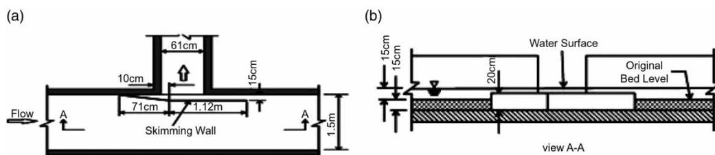
Figure 1 | (a) Plan and (b) cross-section of the skimming wall (Barkdoll *et al.* 1999).
