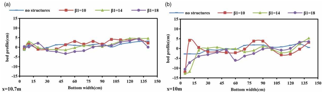
**Figure 9** | Transverse profile of bed in main channel in (a) lower and (b) upper openings with and without structure.
