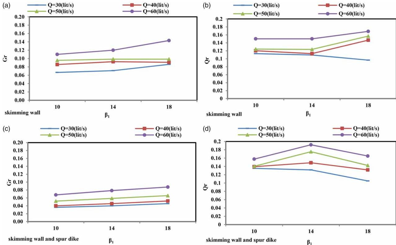
Figure 7 | Relation of skimming wall angle, sediment ratio and discharge entering the intake.
