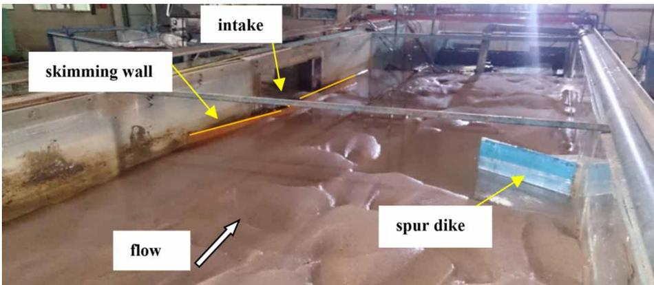
Figure 3 | A schematic of the flume, intake, spur dike and skimming wall.
