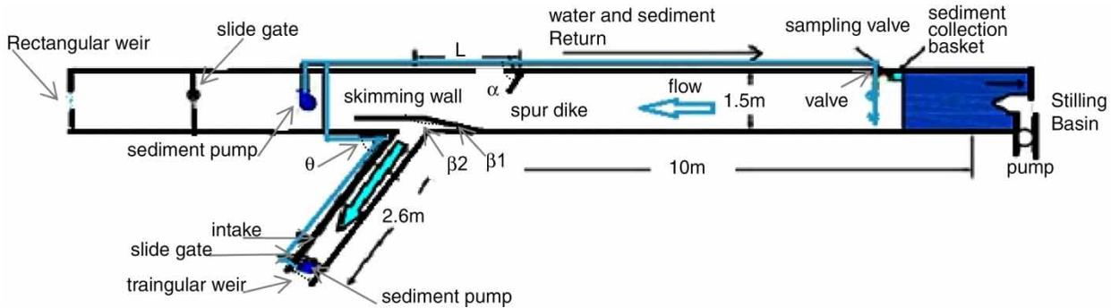
Figure 2 | A schematic of the flume, spur dike, skimming wall and water circulation system and sediment.
