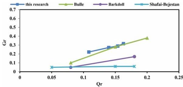
**Figure 11** | Comparing results of diverted sediment ratio in this study with results of other studies in the no-structure state of sediment control.
