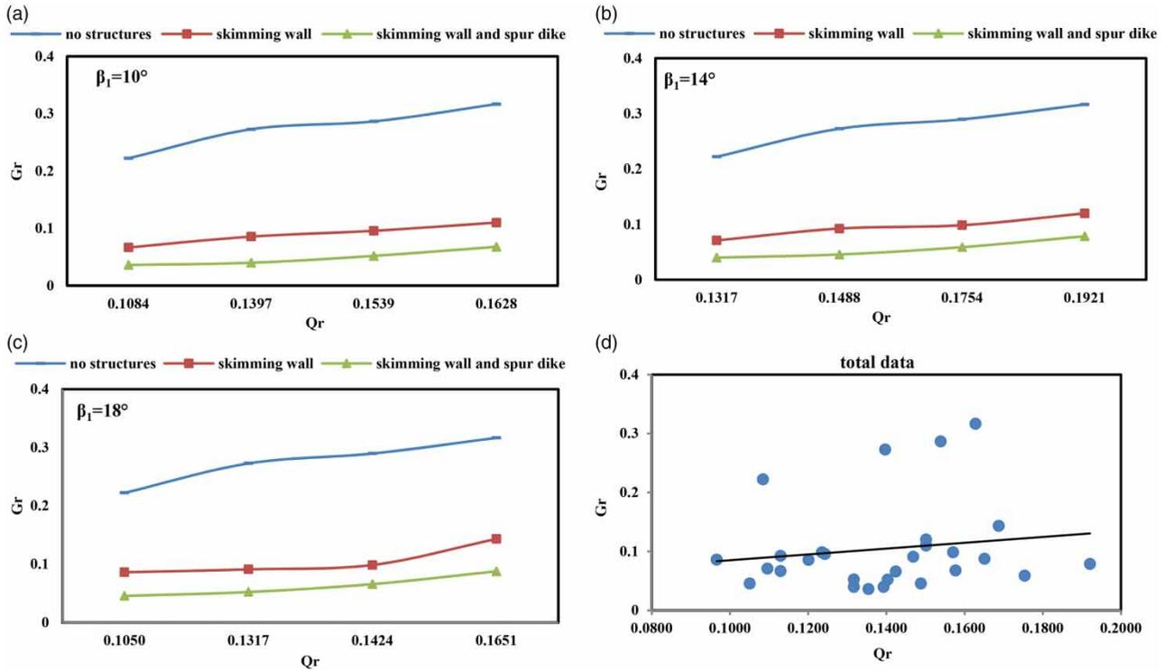
**Figure 5** | Ratio of diverted sediment into the intake in terms of ratio of intake discharge, for angles between the skimming wall and bank of (a)  $10^\circ$ , (b)  $14^\circ$ , and (c)  $18^\circ$ , and (d) total data.
