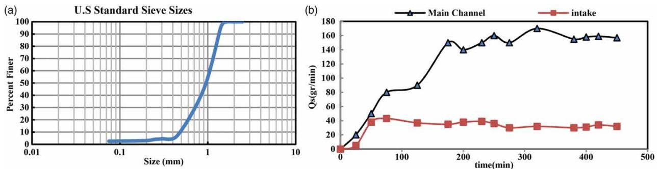
Figure 4 | (a) Grading diagram of sediments; (b) sediment discharge changes in time.
