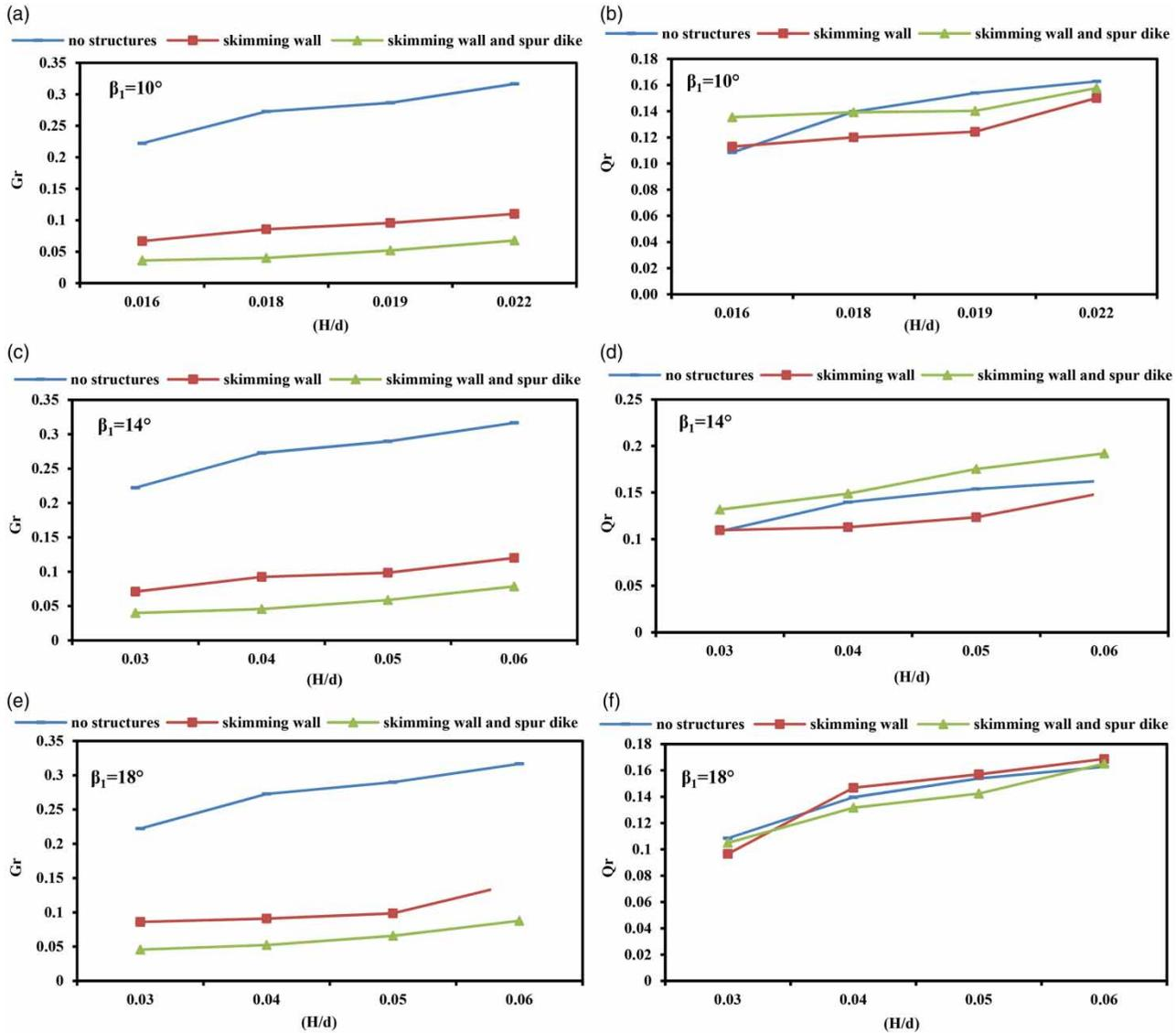
**Figure 6** | Ratio of flow depth to out-of-bed height of the skimming wall to diverted sediment into the intake.
