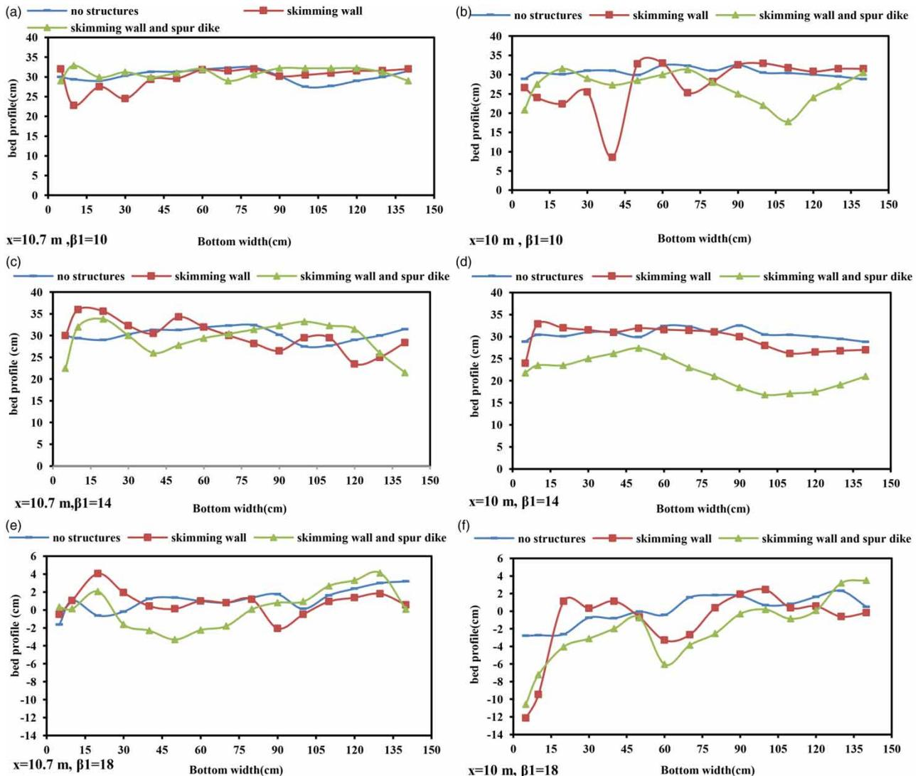
**Figure 10** | Transverse profile of bed in main channel in lower (a), (c), (e) and upper (b), (d), (f) openings with and without structure.
