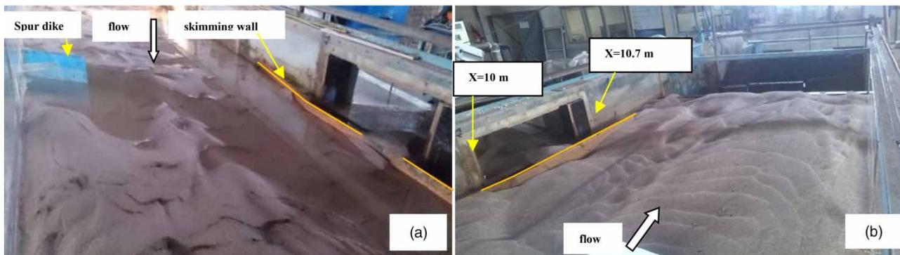
Figure 8 | Skimming wall and sediments accumulated in front of the intake entrance.
