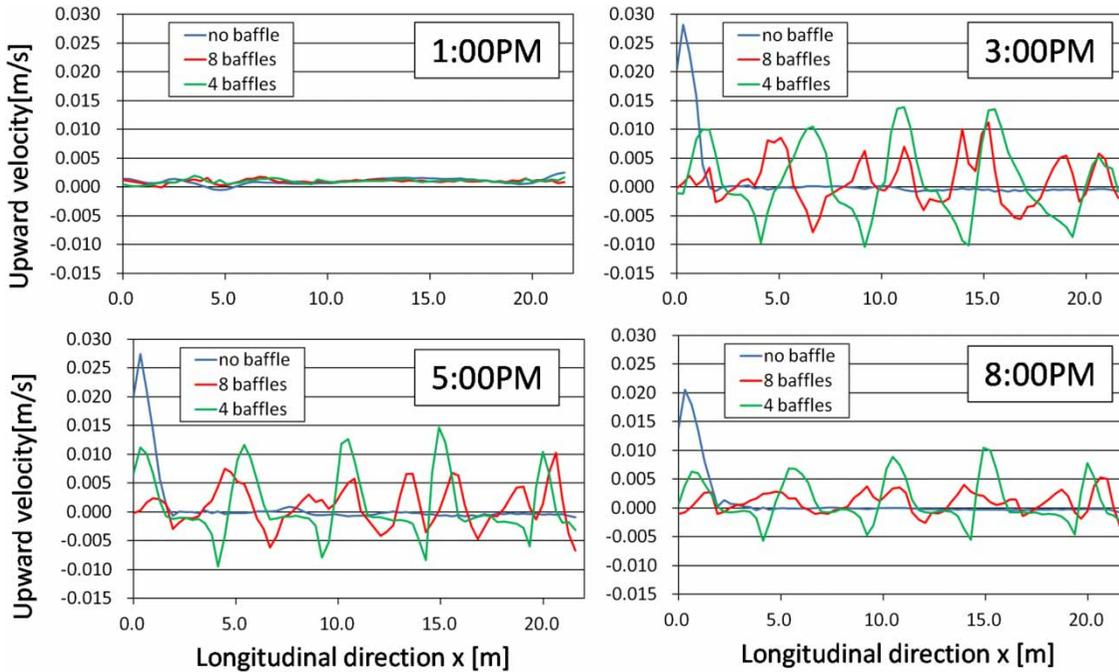
Figure 9 | Calculated average axial velocity distribution [m/s] in the longitudinal direction [m]. Graphs show distributions at 1:00, 3:00, 5:00, and 8:00 PM.
