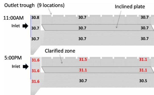
Figure 2 | Measured temperature distributions (°C) in the sedimentation basin at 11:00 AM and 5:00 PM.
