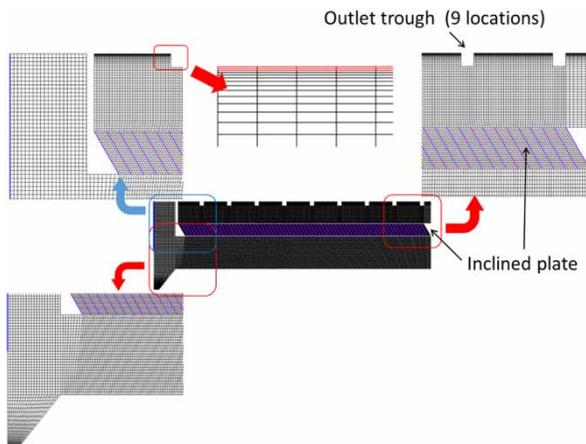
Figure 4 | Boundary conditions of CFD.
