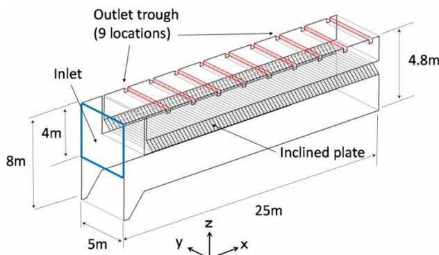
Figure 3 | Calculation model of the sedimentation basin for CFD.
