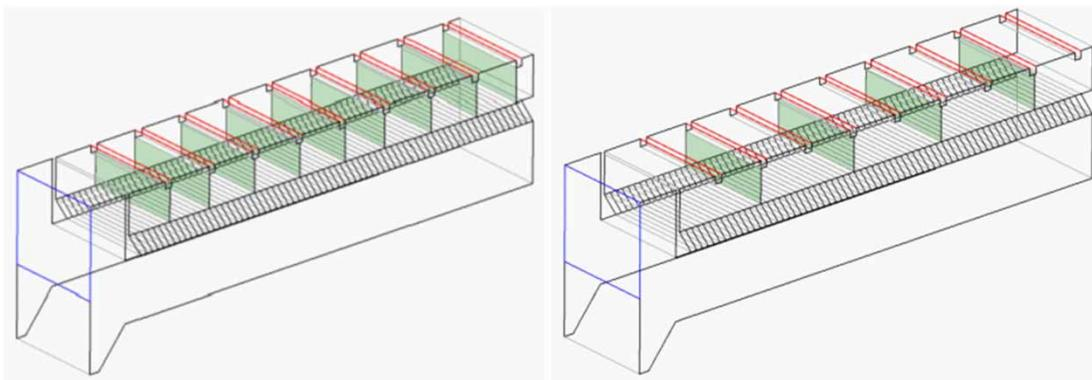
Figure 6 | Calculation model using baffle plates in two cases.
