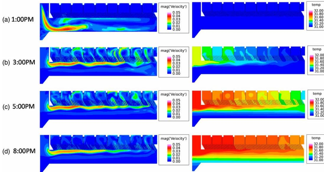
**Figure 8** | Calculated transient velocity and temperature contours in the sedimentation basin using eight baffle plates.
