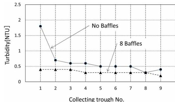
Figure 10 | Measured turbidity at each collecting trough. Circles show the case of no baffle plate, and triangles the case of eight baffle plates.
