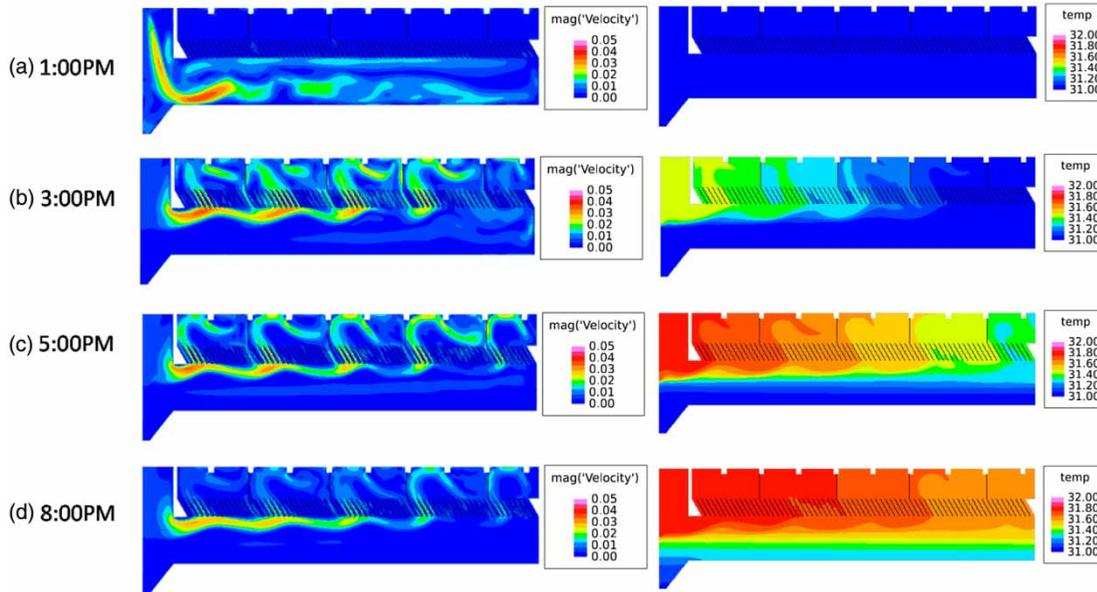
**Figure 7** | Calculated velocity and temperature contours in the sedimentation basin using four baffle plates.
