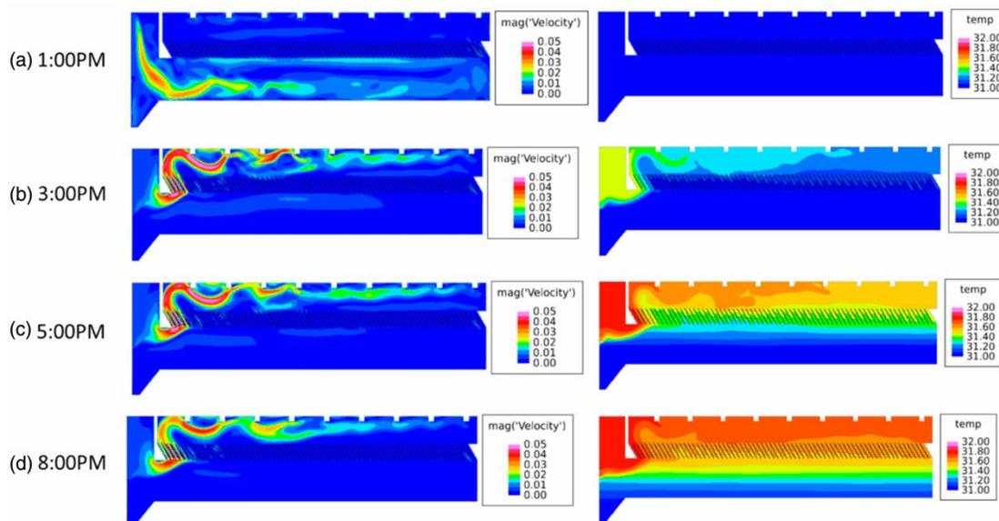
Figure 5 | Calculated transient velocity and temperature contours in the sedimentation basin.
