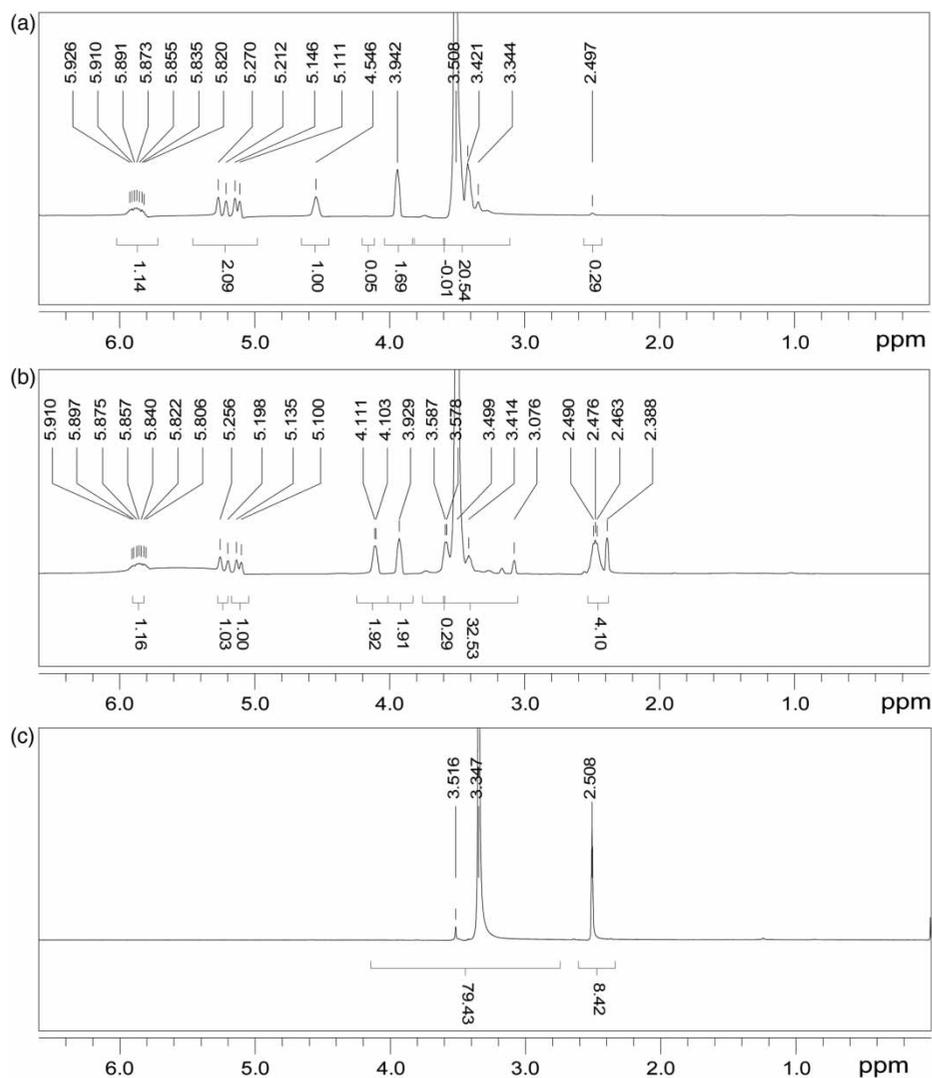
Figure 3 |  $^1H$ -NMR spectra of (a) APEG, (b) APEL and (c) AA-APEL.
