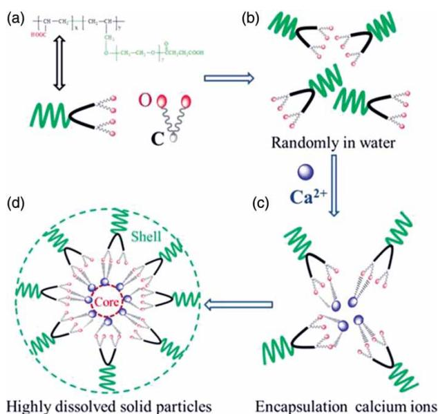
**Figure 8** | Encapsulation route of calcium ions via carboxyl groups.
