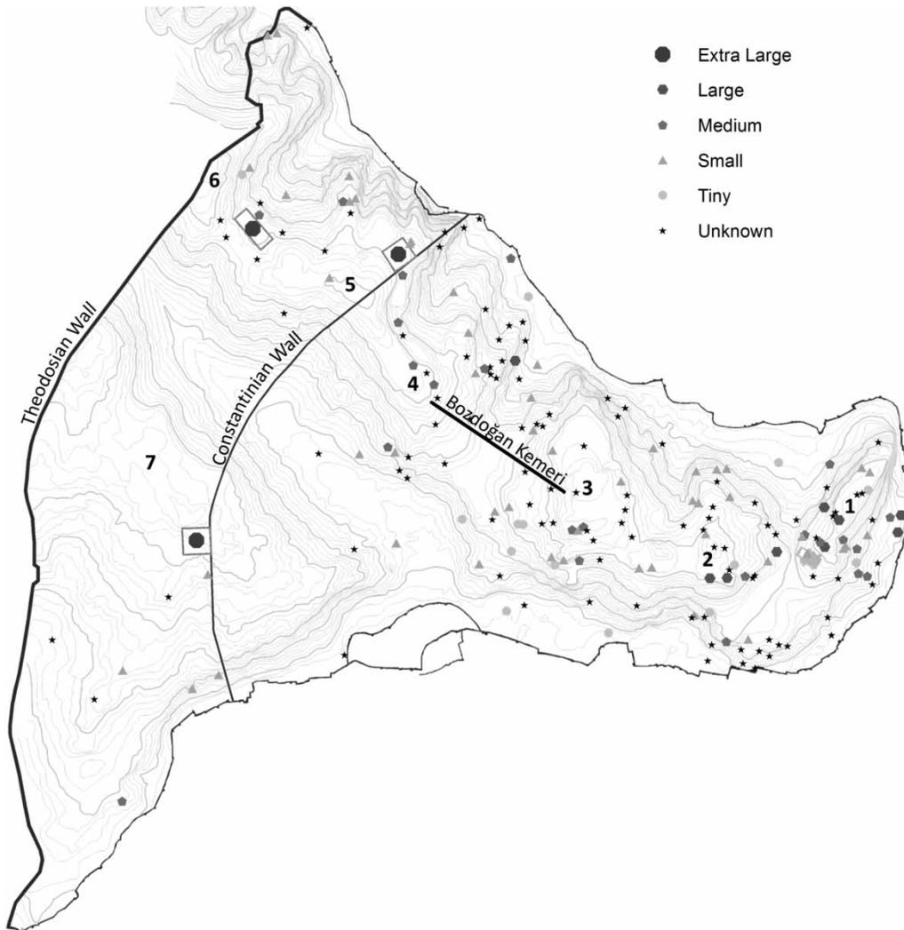
**Figure 2** | The city's 211 cisterns categorised by volume: Extra Large >100,000 m<sup>3</sup>; Large 5,000–99,999 m<sup>3</sup>; Medium 1,000–4,999 m<sup>3</sup>; Small 100–999 m<sup>3</sup>; Tiny <100 m<sup>3</sup>. Numbers indicate the hills of the city.
