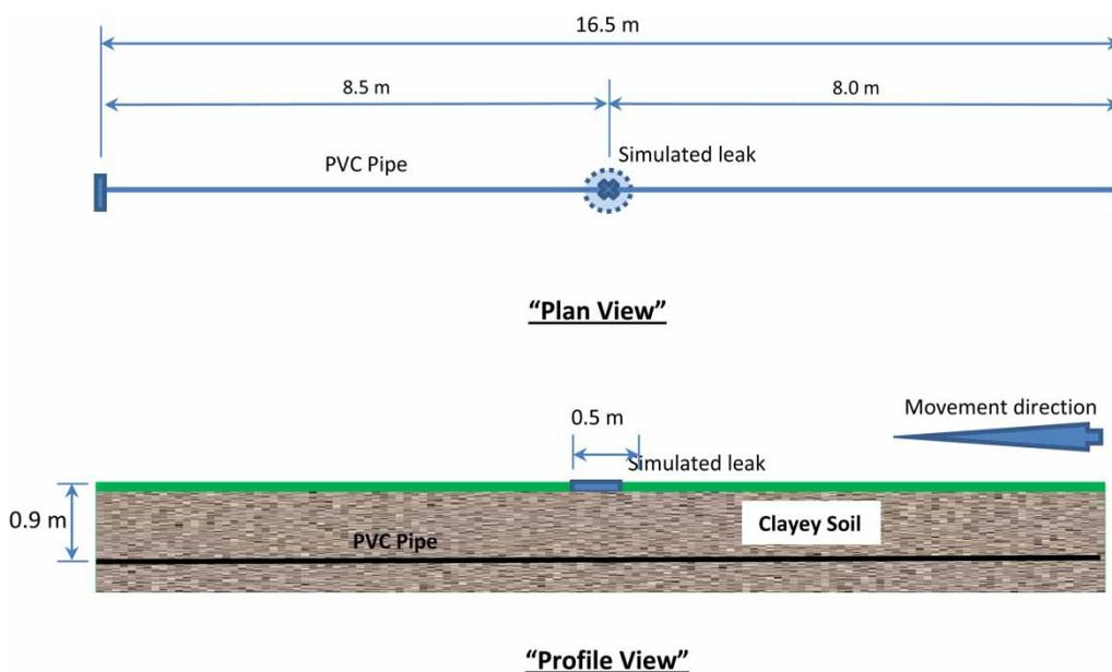
**Figure 2** | Simulated leak experimental layout.
