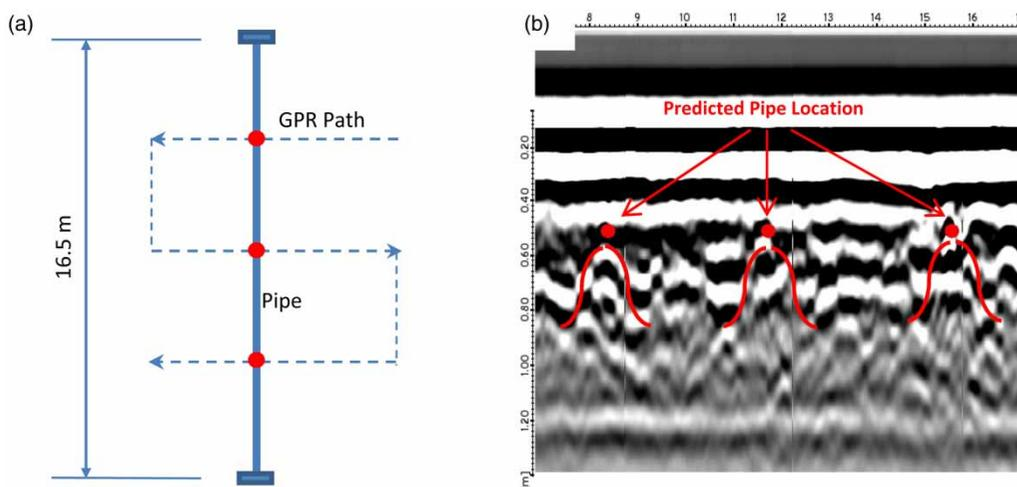
**Figure 3** | (a) Path of the GPR on top of the buried pipe; (b) profile of the subsurface using the MALÁ ground penetrating radar (GPR) equipped with the 500 MHz shielded antenna, location of the pipe is indicated by the hyperbola and by the red dots. Please refer to the online version of this paper to see this figure in color: <http://dx.doi.org/10.2166/ws.2017.044>.
