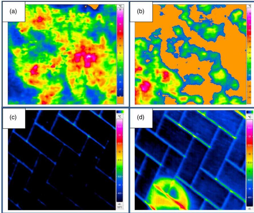
**Figure 4** | (a) IR image for simulated leak case study 'dry location'; (b) IR image for simulated leak case study 'wet location'; (c) IR image for real leak case study 'dry location'; (d) IR image for real leak case study 'wet location'.
