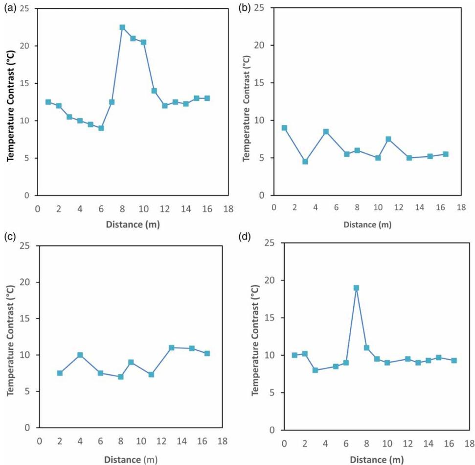
**Figure 5** | (a) Predicted leak locations of the simulated leak case, operating conditions (1); (b) predicted leak locations of the simulated leak case, operating conditions (2); (c) predicted leak locations of the simulated leak case, operating conditions (3); (d) predicted leak locations of the simulated leak case, operating conditions (4).
