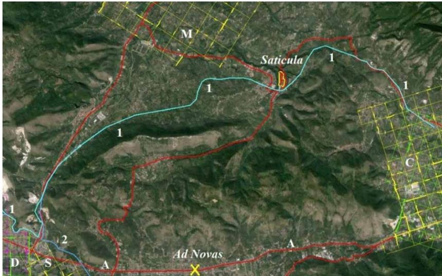
**Figure 7** | The initial parts of Carmignano and *Aqua Iulia* aqueducts. 1: First part of *Aqua Iulia* and Carmignano aqueducts, and then only *Aqua Iulia*; 2: beginning of the subsequent section of Carmignano aqueduct; A: *via Appia*; C: part of the centuriations (land divisions) *Caudium I* and *Caudium II*; S: part of the centuriation of *Suessula*; M: part of the centuriation of the middle *Volturno River*; D: part of the centuriations *Ager Campanus I* and *Ager Campanus II*.
