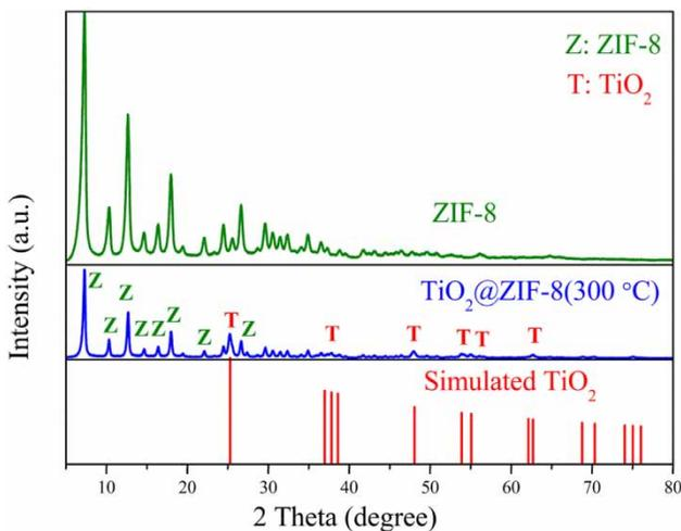
**Figure 2** | XRD patterns of TiO<sub>2</sub>@ZIF-8 calcined at 300 °C, ZIF-8, and simulated TiO<sub>2</sub> (PDF21-1272).
