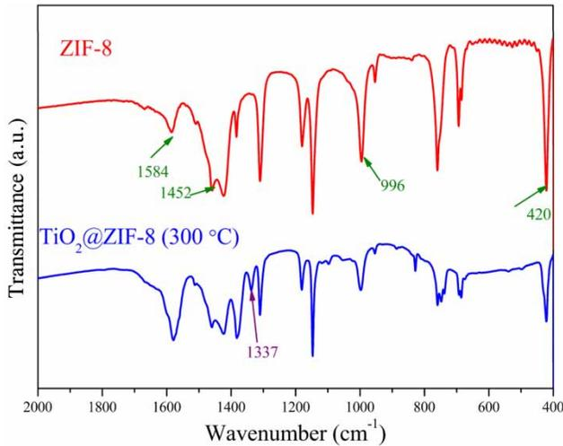
Figure 4 | FT-IR spectra of ZIF-8 and TiO<sub>2</sub>@ZIF-8 (300 °C).
