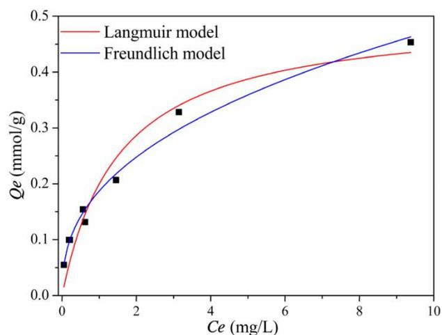
**Figure 6** | Adsorption isotherms of As(III) on TiO<sub>2</sub>@ZIF-8 in dark conditions. Initial As(III) concentration range from 0.2 to 10 mg/L, pH 7.0, solid/solution ratio of 0.04 g/L, and  $T = 25 \pm 1$  °C.
