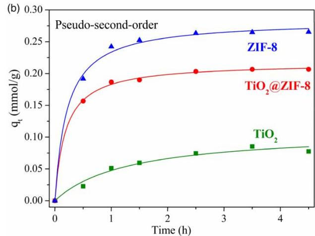
Figure 5 | Adsorption kinetics of As(III) on TiO<sub>2</sub>, ZIF-8, and TiO<sub>2</sub>@ZIF-8 in dark conditions: pseudo-first-order (a), pseudo-second-order (b); the initial As(III) concentration of 2 mg/L, pH 7.0, solid/solution ratio of 0.04 g/L, and T = 25 ± 1 °C.
