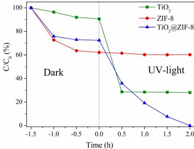
**Figure 8** | Effect of As(III) removal with different materials.  $C_0$  of 2 mg/L, pH 7.0, solid/solution ratio of 0.04 g/L.
