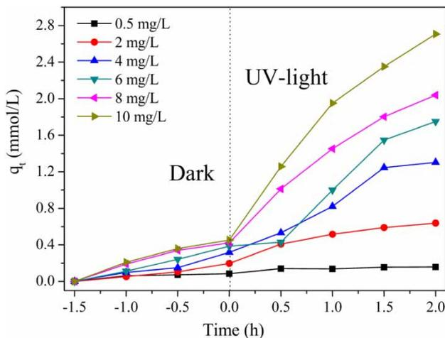
**Figure 9** | Effect of the different initial concentrations on the removal of As(III). pH 7.0, solid/solution ratio of 0.04 g/L.
