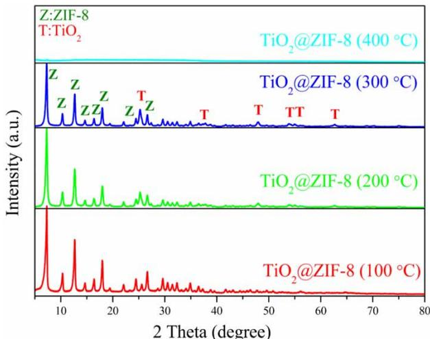
**Figure 1** | XRD patterns of TiO<sub>2</sub>@ZIF-8 at the different calcination temperatures. The diffraction peaks of the TiO<sub>2</sub> phase are marked with T, and the diffraction peaks of the ZIF-8 phase are marked with Z.
