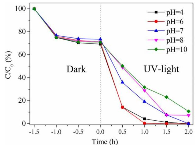
**Figure 10** | Effect of As(III) removal in samples under different pH conditions.  $C_0$  of 2 mg/L, solid/solution ratio of 0.04 g/L.
