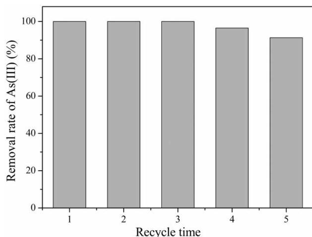
**Figure 11** | Influence of reutilization cycles for the removal rate of As(III).
