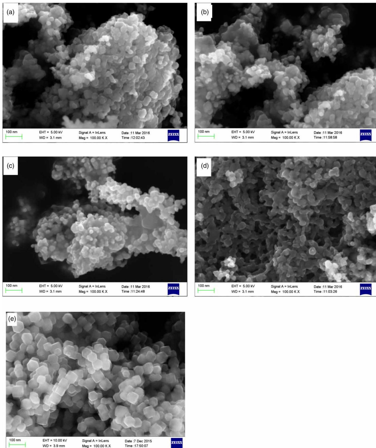
**Figure 3** | SEM images for TiO<sub>2</sub>@ZIF-8 with the different calcination temperatures: (a) 100 °C; (b) 200 °C; (c) 300 °C; (d) 400 °C; and (e) ZIF-8.
