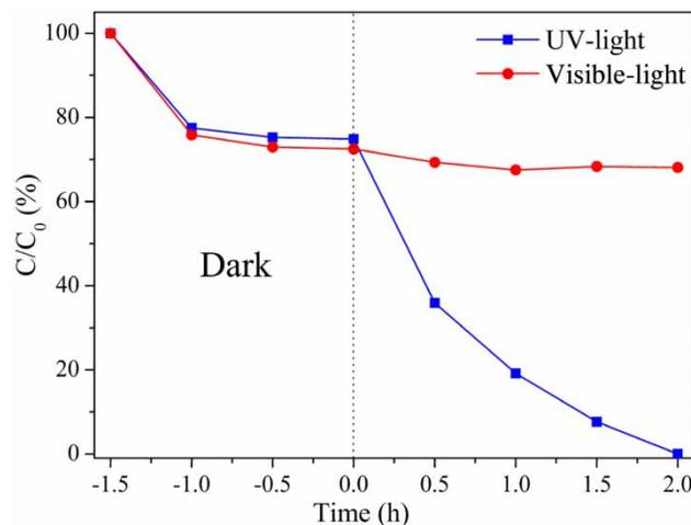
**Figure 7** | Effect of illumination condition on the removal of As(III).  $C_0$  is the initial concentration of As(III), and  $C$  is the concentration of As(III) at different reaction times.  $C/C_0$  represents the ratio  $C$  to  $C_0$ .  $C_0$  of 2 mg/L, pH 7.0, solid/solution ratio of 0.04 g/L.
