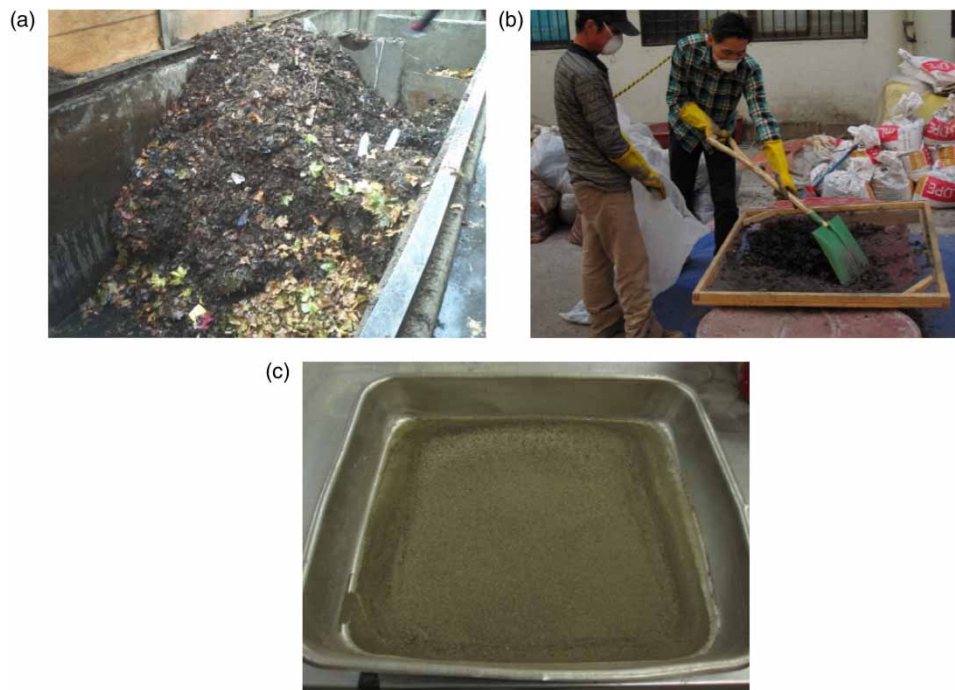
Figure 2 | Preparation of dry sample of non-point source pollutants: (a) collection of non-point source pollutants, (b) first sieve separation, and (c) dry sample of non-point source pollutants after second sieve separation.
