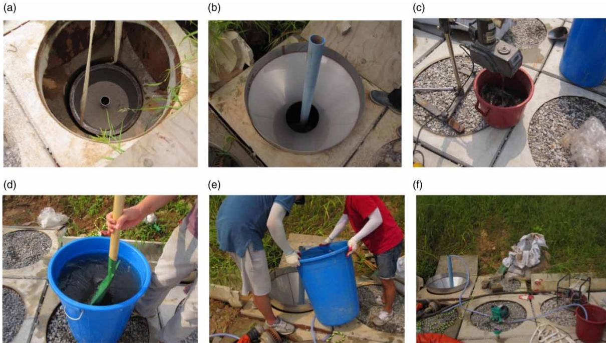
**Figure 15** | Field test procedure to evaluate filtration efficiency of sand filter layer: (a) installing sand filter layer into infiltration well, (b) setting floating device and outflow pipe, (c) mixing non-point source pollutants sample with water, (d) preparing artificial urban runoff with non-point source pollutants, (e) pouring artificial urban runoff into infiltration well, and (f) monitoring outflow.
