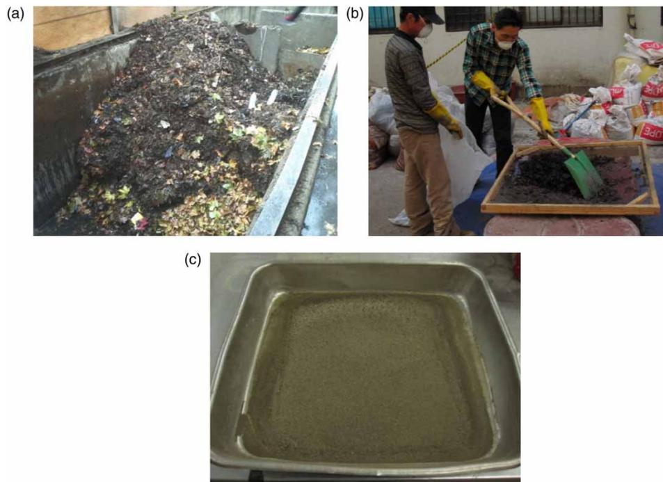
**Figure 2** | Preparation of dry sample of non-point source pollutants: (a) collection of non-point source pollutants, (b) first sieve separation, and (c) dry sample of non-point source pollutants after second sieve separation.
