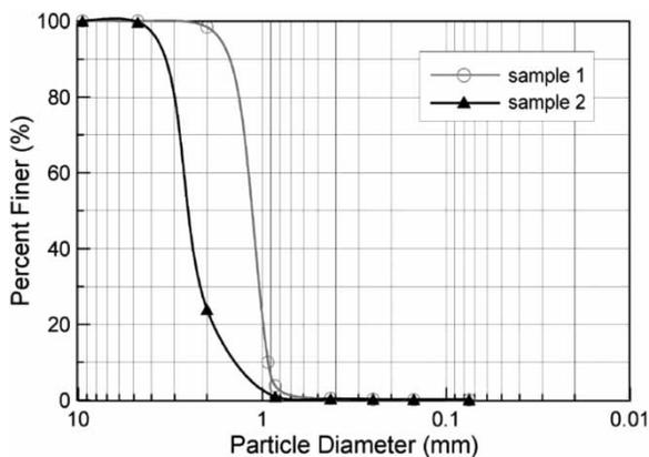
**Figure 4** | Grain size distribution curves for filter layers (sample 1 and sample 2).**Table 4** | Material properties of sand filter layers (sample 1 and sample 2)
