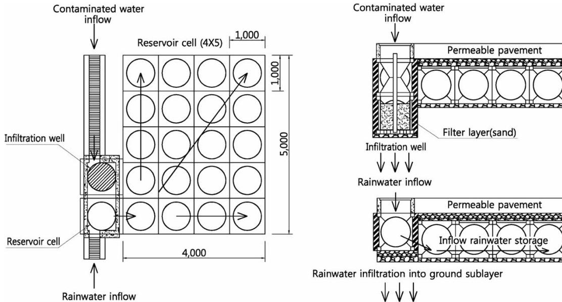
Figure 13 | Conceptual diagrams of pilot-scale rainwater reservoir.
