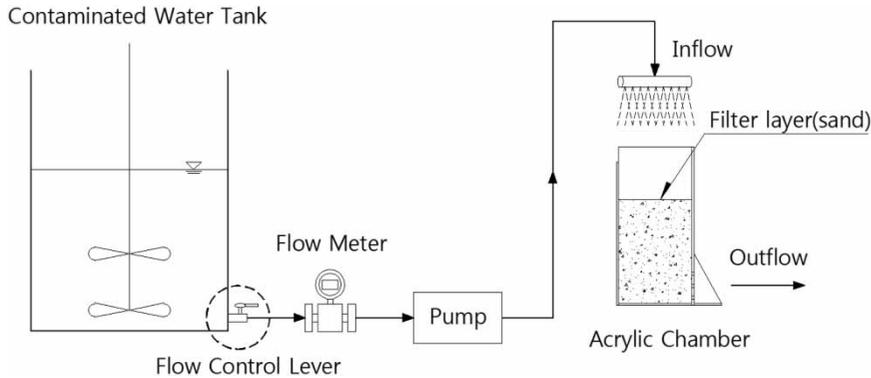
Figure 5 | Schematic diagram of laboratory-scale chamber system.
