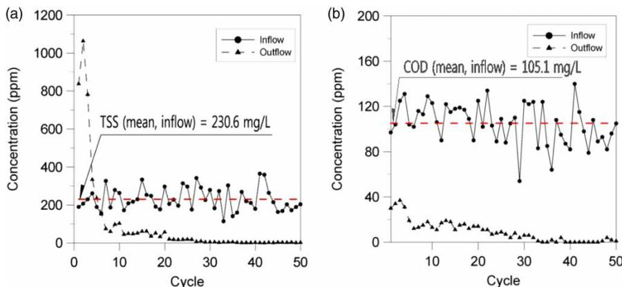
**Figure 16** | Measurement of TSS and COD with testing cycles: (a) TSS and (b) COD.
