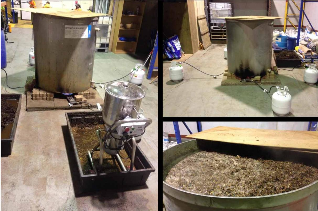
**Figure 2** | 'Tea' brewing setup with blender, brewing tank and gas burners.
