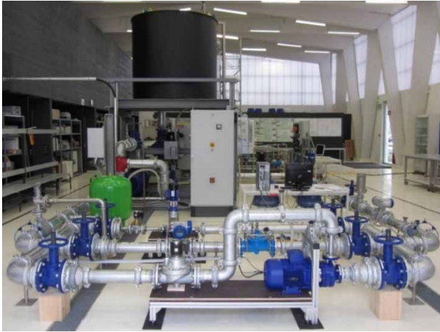
Figure 3 | Testing plant at the UniBwM. It comprises a combination of feeding pumps and regulating valves, for generating a wide range of flows and pressures, and different measuring devices (pressure sensors and flow meters).
