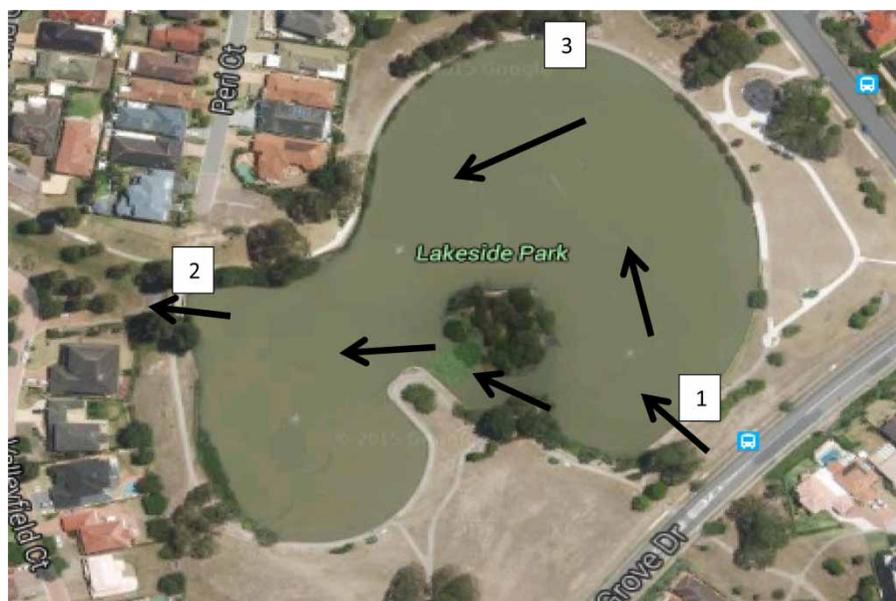
**Figure 1** | Wattle Grove Lake. Point 1 is the inlet and Point 2 is the outlet. Point 3 was sampled as an extra point for statistical reasoning (average and standard deviation). The flow is shown using the arrows (Google Maps 2016).
