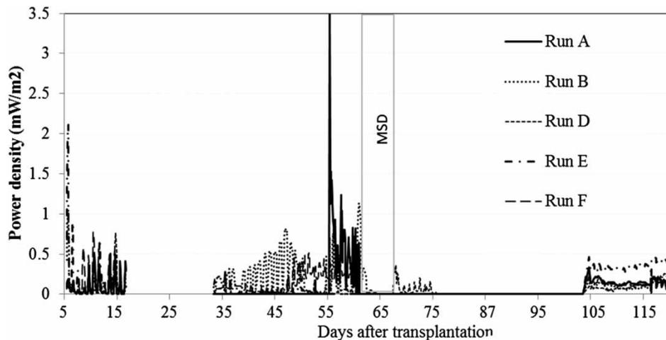
**Figure 6** | Power density from the PF-MFCs. MSD means midsummer drainage to dry up the soil layers. F indicates a period from days 16 to 30 after transplantation, which data could not be obtained due to technical difficulties in the logger.
