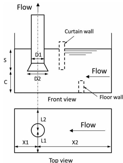
Figure 4 | Geometrical parameters in a typical pump intake system.
