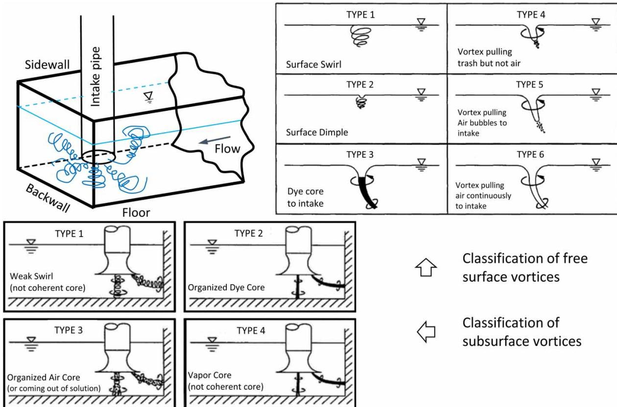
**Figure 1** | Schematics of a typical pump intake system and classification of vortices (the difference between free surface and subsurface vortices is the location where they originate) (adapted from ANSI/HI 9.8 2012).
