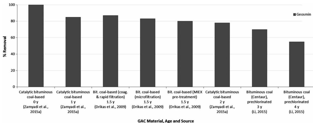
**Figure 6** | Impact of age on geosmin removal efficiency of GAC with an EBCT of 4–5 min.
