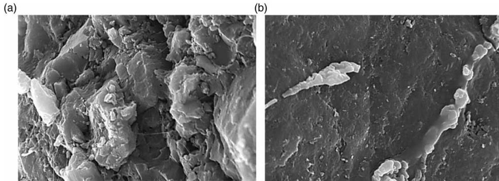
**Figure 3** | GAC surface observation using scanning electron microscopy (SEM –  $\times 5,000$ ): (a) new carbon (less than 5,000 bed volume) and (b) aged carbon (over 90,000 bed volume) (Images' copyright: A. Zamyadi).
