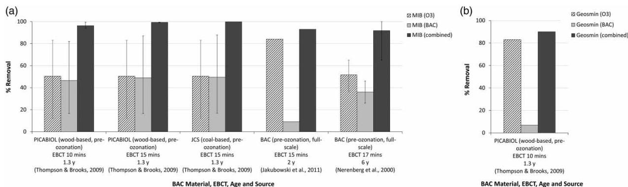
Figure 4 | Contribution of both ozonation and bio-filtration to removal of (a) MIB and (b) geosmin in O<sub>3</sub>/BAC systems.
