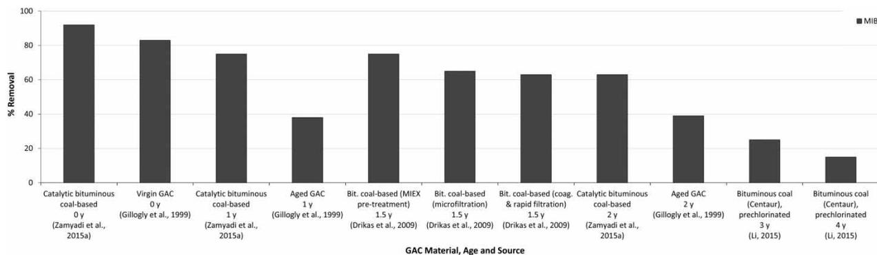
Figure 5 | Impact of age on MIB removal efficiency of GAC with an EBCT of 4–5 min.
