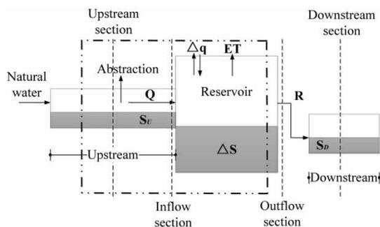
Figure 1 | Generalized structure of a reservoir (where  $Q$  and  $R$  are the reservoir inflow and reservoir release,  $\Delta q$  is the difference between local inflow and water withdrawal,  $ET$  is the evapotranspiration,  $\Delta S$  is the storage variation;  $S_u$  is the initial water volume in the upstream section; and  $S_D$  is the initial water volume in the downstream section, respectively).
