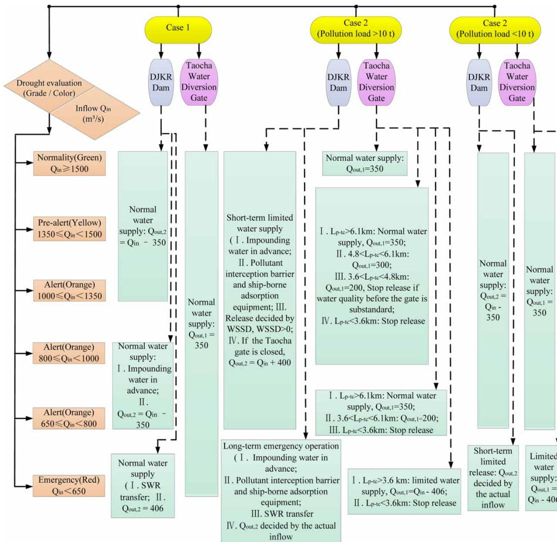
**Figure 6** | Generalized emergency operation rules ( $L_{p-tc}$  is the distance between the pollution point and the Taocha water diversion gate;  $Q_{in}$  is the monthly inflow of DJKR,  $m^3 s^{-1}$ ;  $Q_{out,1}$  is the release at the Taocha gate,  $m^3 s^{-1}$  and  $Q_{out,2}$  is the release of DJKR,  $m^3 s^{-1}$ , respectively).
