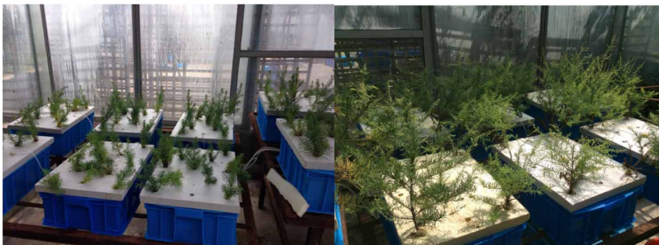
Figure 1 | Floating mat Suaeda salsa -based treatment systems.
