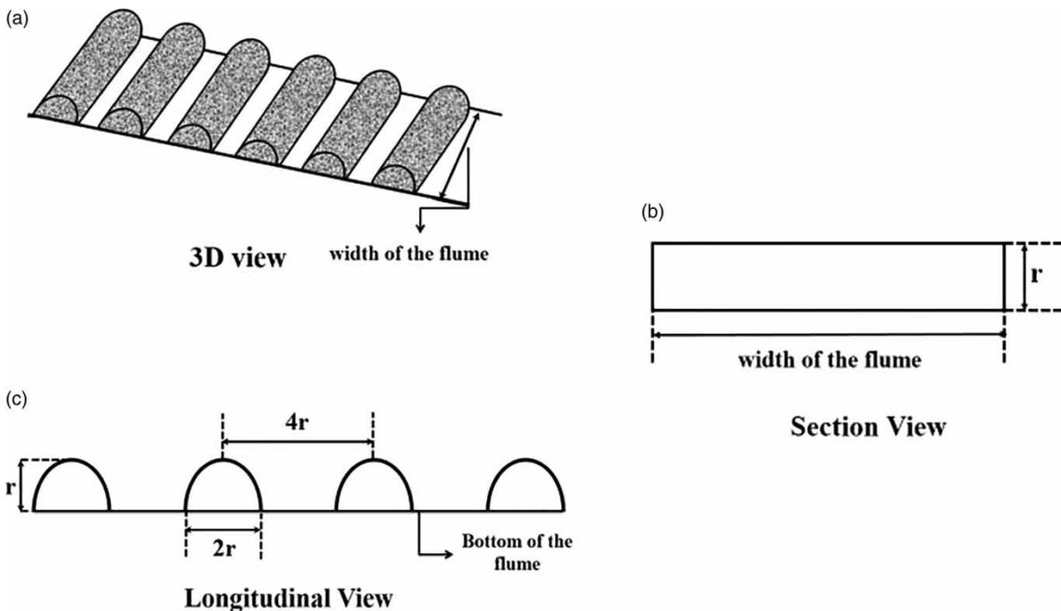
**Figure 4** | Schematic view of the corrugated bed of the stilling basin: (a) 3D view, (b) section view, (c) longitudinal view.
