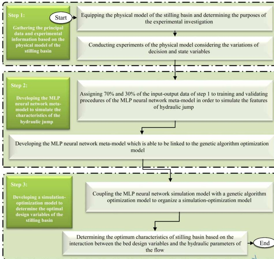
**Figure 1** | Framework of the proposed data-driven simulation-optimization methodology for optimal design of stilling basin features with adverse slope and corrugated bed.
