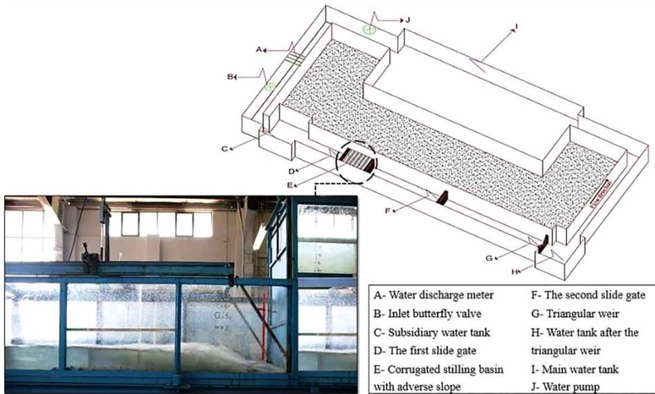
**Figure 3** | The experimental flume with stabilized hydraulic jump on the corrugated bed with adverse slope.
