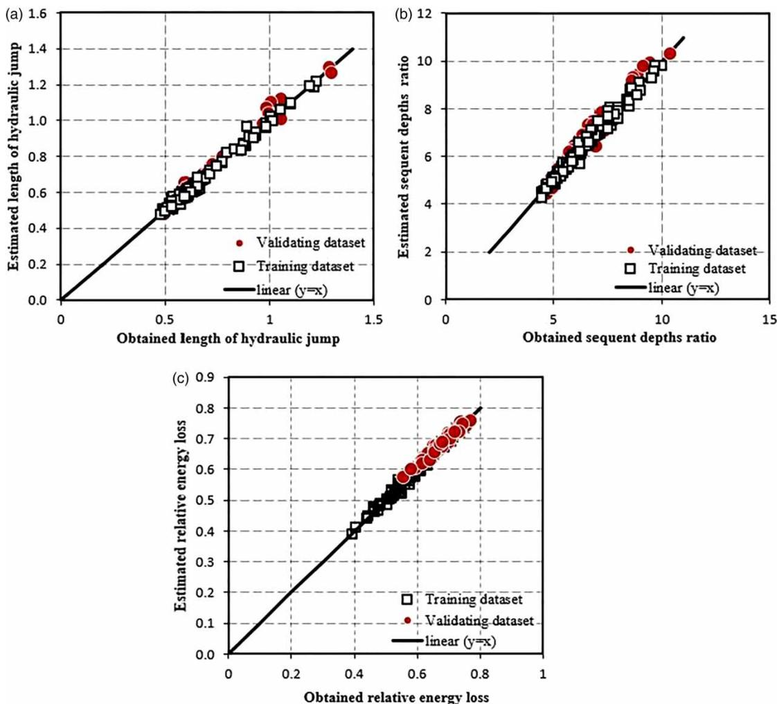
**Figure 5** | The results of the developed MLP neural network models to estimate (a) length of the hydraulic jump, (b) the sequent depths ratio, (c) the relative energy loss of the flow for training and validating datasets.
