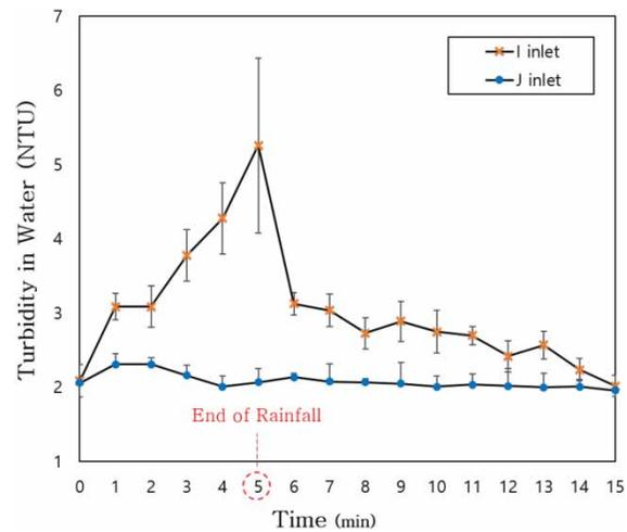
**Figure 2** | Comparison of turbidity before and after rainfall for I-type and J-type inlet pipes.
