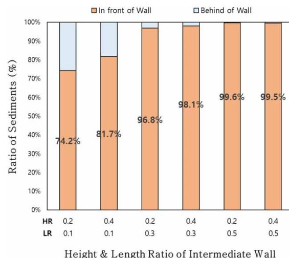
**Figure 3** | Changes in the ratio of sediment in front of and behind the intermediate wall with variable distance and height ratios.
