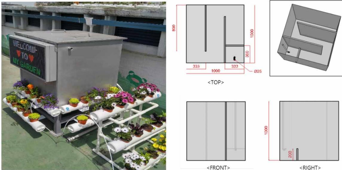
**Figure 5** | Prototype rainwater tank used for the for field scale tests.
