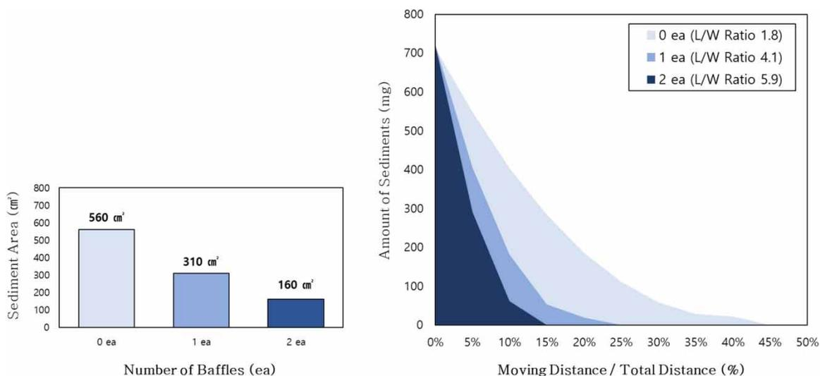
**Figure 4** | Sediment settling area and volume according to the number of baffles.
