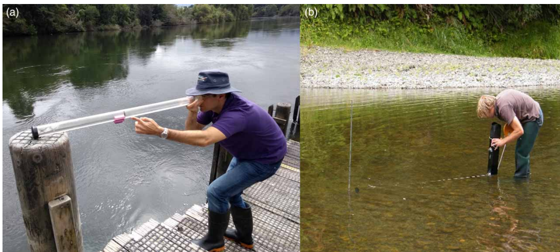
Figure 1 | Measurement of visual water clarity in New Zealand. (a) The SHMAK clarity tube in use for water of relatively low clarity. The black target (20 mm diameter disc) is mounted on an aquarium magnet that is being moved to the extinction distance. (b) Visual clarity measurement in situ as the horizontal sighting range of a black disc. The observer is using an underwater periscope to observe the extinction distance of the black disc target fixed to a steel stake driven into the streambed (at left) (Photo credits: A. Rob Davies-Colley; B. Graham Timpany).
