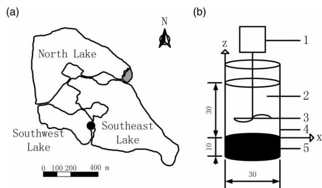
**Figure 1** | (a) Location of sampling in Xuanwu Lake; (b) sketch of the model (cm): 1. motor; 2. overlying water; 3. propeller; 4. Plexiglas cylinder; 5. sediment.
