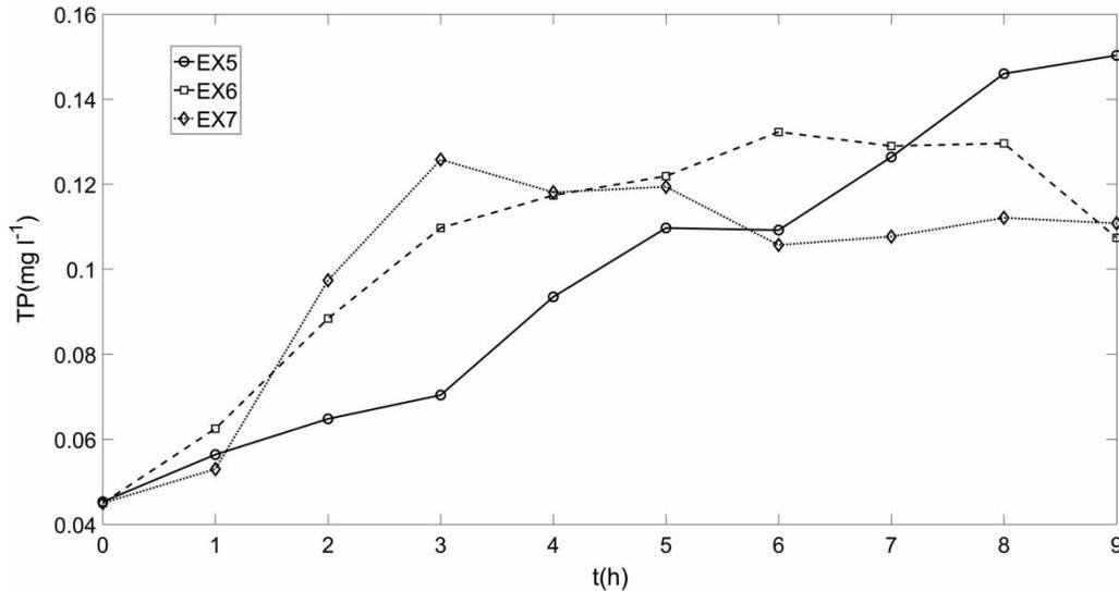
Figure 3 | Variations of TP release rate with different shear velocities.
