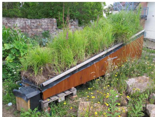
**Figure 1** | Experimental set-up with helophyte mat, at the end of three months in service treating greywater (photograph: A. Zehndorf).
