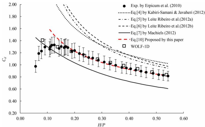
**Figure 3** | Comparison of discharge coefficients for various formulas and the experimental results from Erpicum *et al.* (2010).
