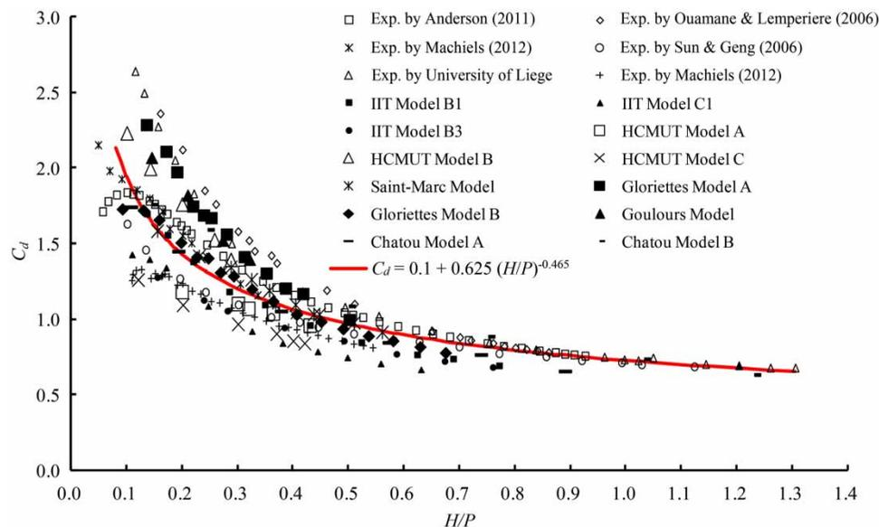
Figure 1 | Relationships of PKW discharge coefficients obtained from various tests and  $H/P$  values.
