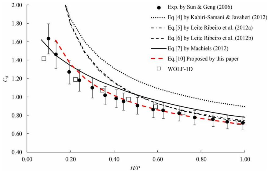
**Figure 2** | Comparison of discharge coefficient for various formulas and the experimental results from Sun & Geng (2006).
