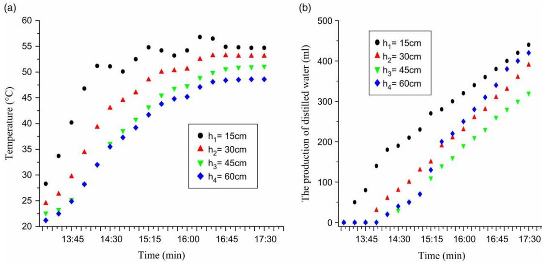
Figure 2 | Variation of (a) temperature and (b) productivity of distilled water versus time for the solar still with four stages.
