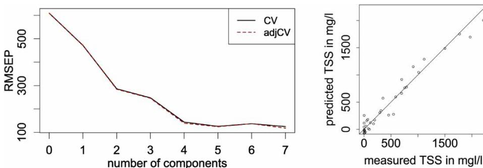
**Figure 2** | Results from the PLS regression using combined mesocosm data from sunny and overcast conditions. Left: The RMSEP against the number of components (latent vectors) for cross-validated (CV) and bias-corrected (adjCV) PLS regressions for TSS (mg l<sup>-1</sup>). Right: Measured against PLS-modelled TSS concentrations using five components ( $R^2 = 0.96$ ).
