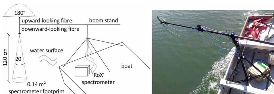
**Figure 1** | Left: Diagram of the boat setup used to acquire reflectance measurements at Passauna drinking water reservoir. Right: Photograph of the system during measurement.
