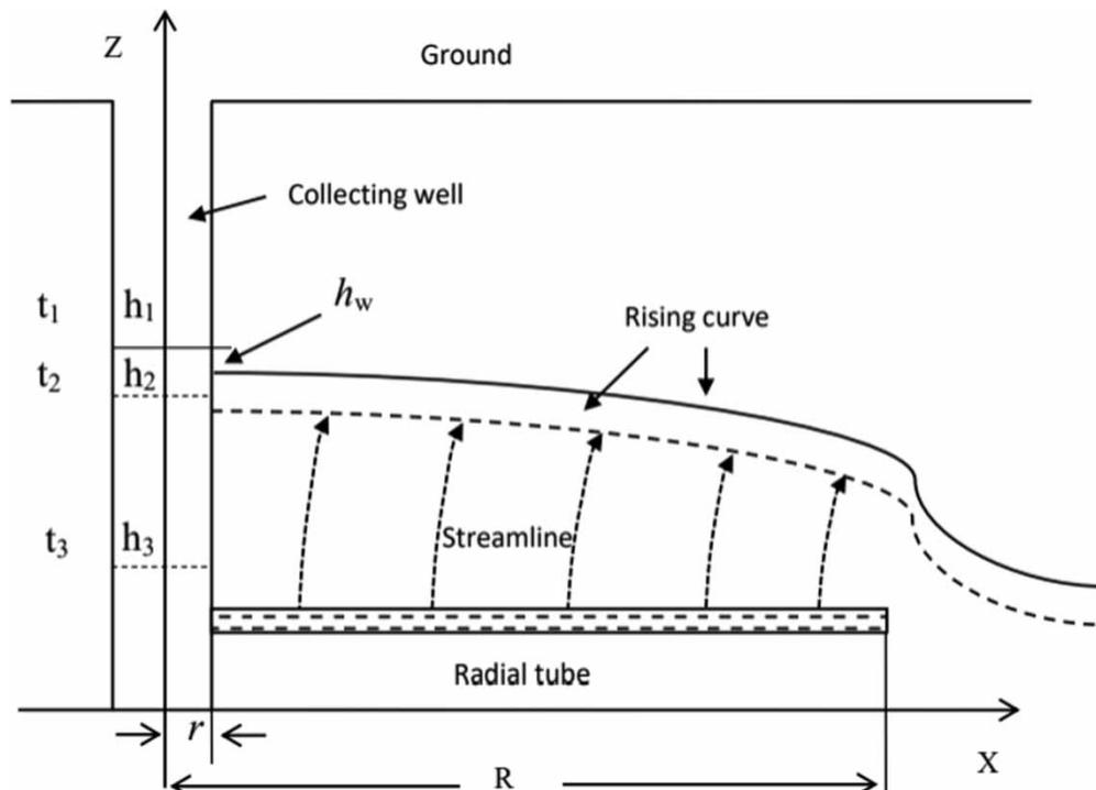
Figure 2 | Schematic diagram of the seepage flow of a radial well in the vertical direction.
